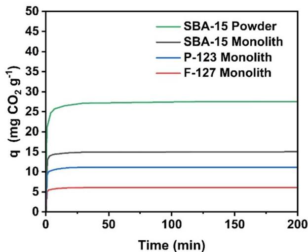
Fig. 4 Pure CO<sub>2</sub> uptake (45 °C, 1 bar) of silica monoliths and SBA-15 powder.
