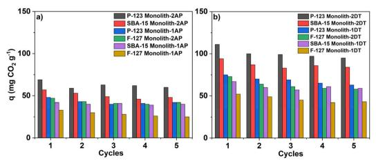
Fig. 9 Cyclic performance of CO<sub>2</sub> adsorption functionalised monoliths with aminosilanes (a) AP and (b) DT.
