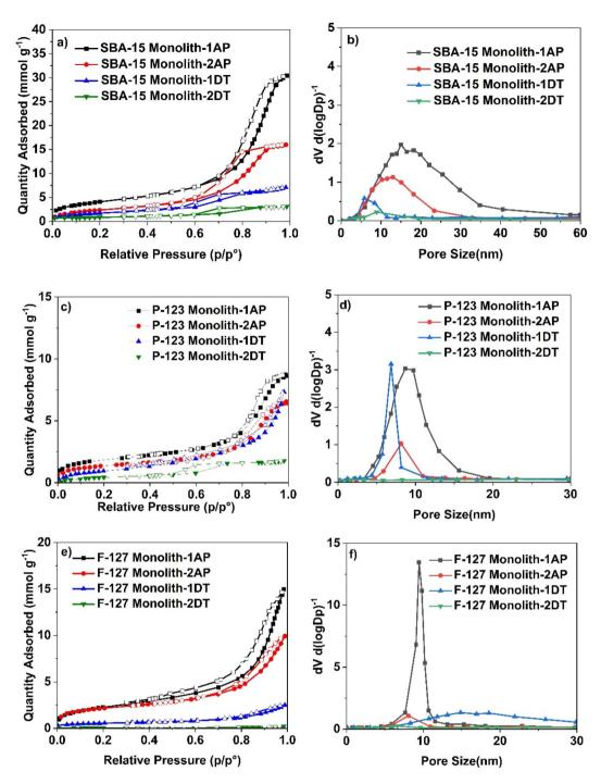
Fig. 5 N<sub>2</sub> adsorption – desorption isotherms at 77 K, and pore size distribution of functionalised (a and b) SBA-15, (c and d) P-123, and, (e and f) F-127 monoliths.
