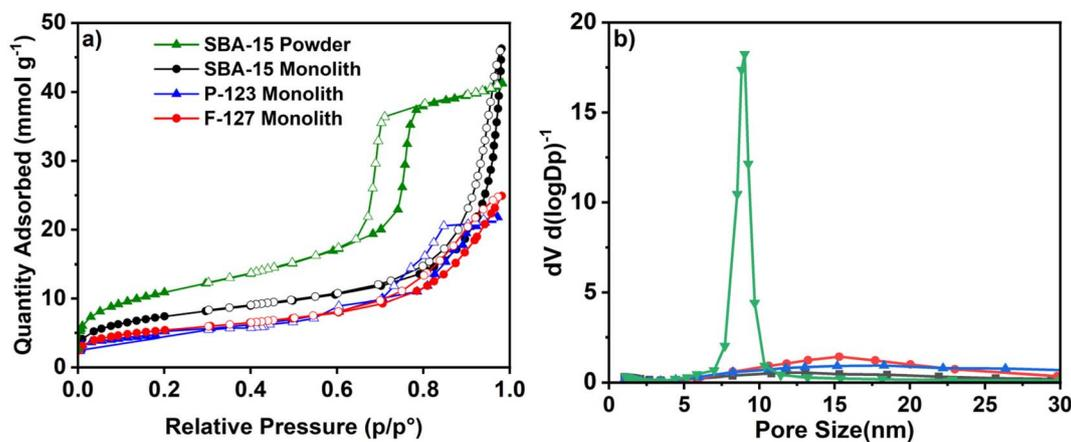
Fig. 3 (a) N<sub>2</sub> adsorption–desorption isotherms at 77 K, and (b) pore size distribution of all monoliths and SBA-15 powder.
