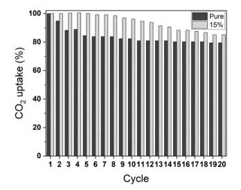
Fig. 10 Cycling stability of  $CO_2$  uptake for P-123 monolith-2DT (45 °C, 1 bar, pure  $CO_2$ ), normalized to the performance of the first cycle (100%).
