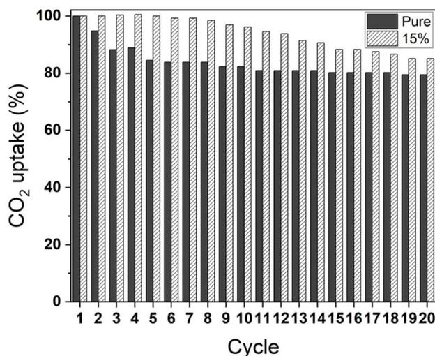
Fig. 10 Cycling stability of CO<sub>2</sub> uptake for P-123 monolith-2DT (45 °C, 1 bar, pure CO<sub>2</sub>), normalized to the performance of the first cycle (100%).
