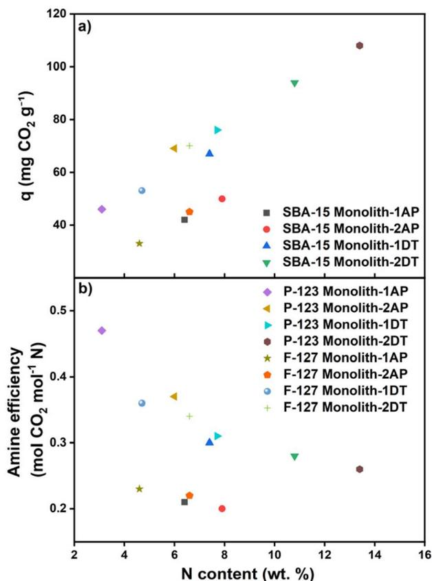
Fig. 7 (a) Adsorption capacity *q* (mg CO<sub>2</sub> per g) at 45 °C and 1 bar, and (b) amine efficiency (mol of CO<sub>2</sub> per mol of N) vs. N content (wt%).
