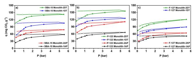
Fig. 8 Pure CO<sub>2</sub> adsorption-desorption isotherms at 45 °C of functionalised monoliths with AP and DT: (a) SBA-15, (b) P-123, and (c) F-127 monoliths.
