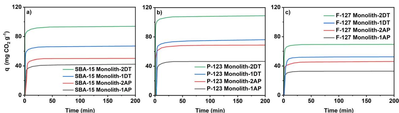
Fig. 6 Pure CO<sub>2</sub> uptake (45 °C, 1 bar) of functionalised monoliths (a) SBA-15, (b) P-123, and (c) F-127 with AP and DT.
