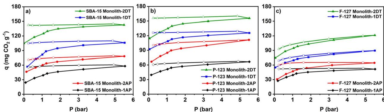
Fig. 8 Pure CO<sub>2</sub> adsorption–desorption isotherms at 45 °C of functionalised monoliths with AP and DT: (a) SBA-15, (b) P-123, and (c) F-127 monoliths.
