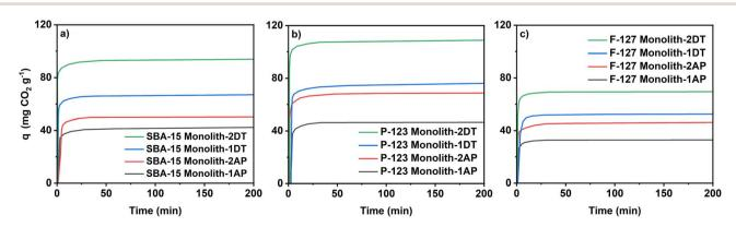
Fig. 6 Pure CO<sub>2</sub> uptake (45 °C, 1 bar) of functionalised monoliths (a) SBA-15, (b) P-123, and (c) F-127 with AP and DT.
