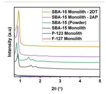
Fig. 2 Powder low angle X-ray diffraction patterns of pure presynthesized SBA-15 powder and monolithic adsorbents.
