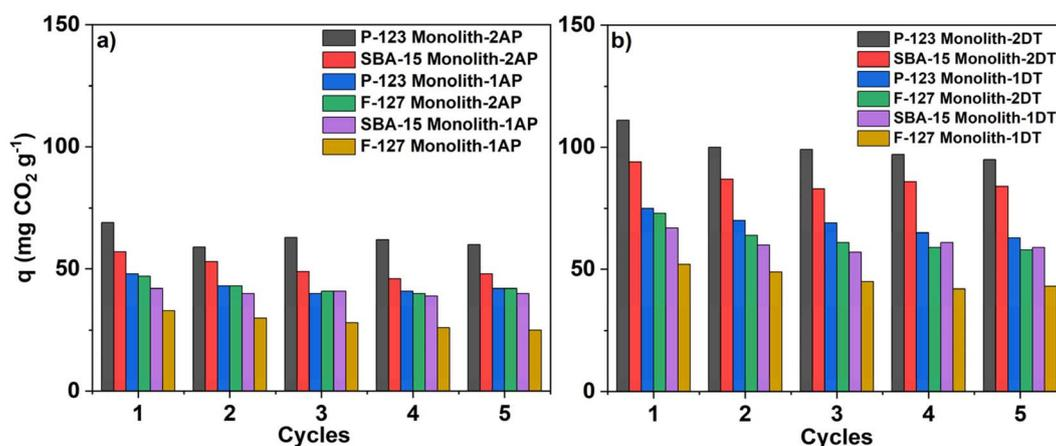
Fig. 9 Cyclic performance of CO<sub>2</sub> adsorption functionalised monoliths with aminosilanes (a) AP and (b) DT.
