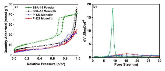
(a)  $N_2$  adsorption–desorption isotherms at 77 K, and (b) pore size distribution of all monoliths and SBA-15 powder.
