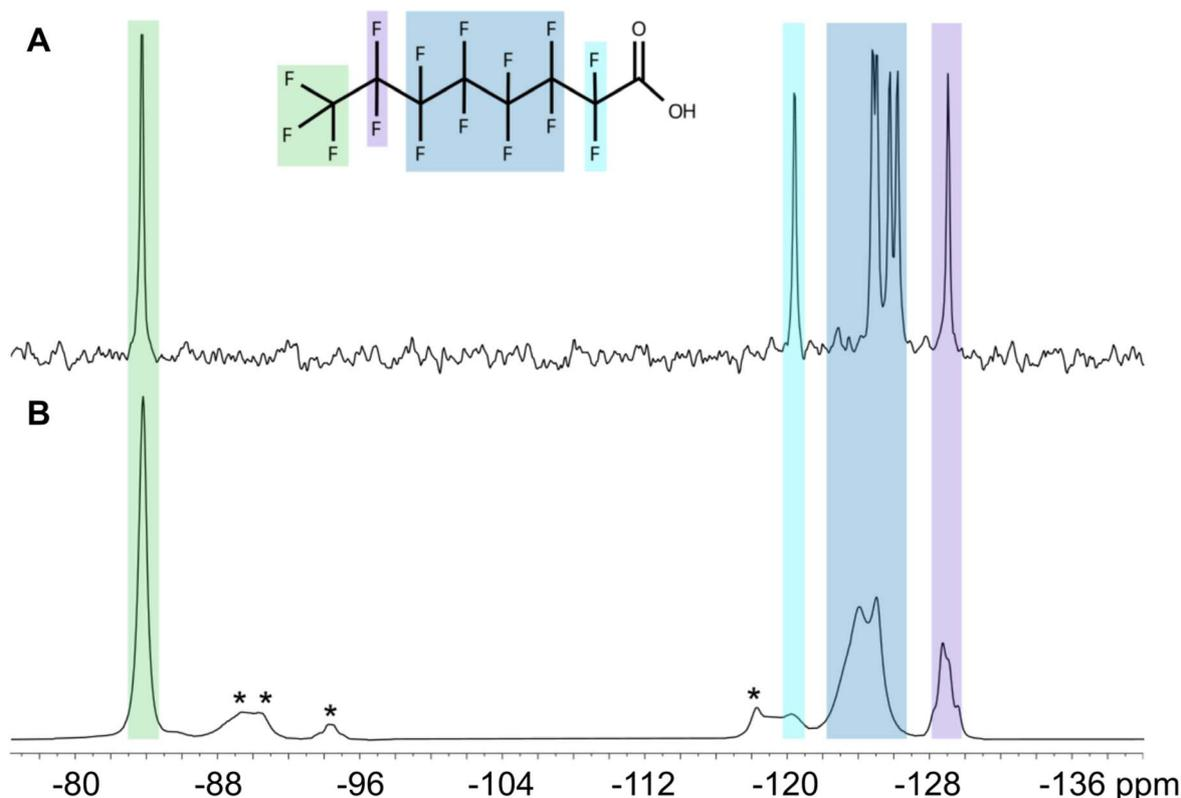
Fig. 1 Representative <sup>19</sup>F spectra of (A) a 50 ppm solution of PFOA (MAS = 4 kHz) and (B) solid PFOA (MAS = 20 kHz). Both spectra were acquired using a 3.2 mm solid-state MAS NMR probe. Spinning sidebands are marked with asterisk. The resonances are colour-coded to match the chemical structure of PFOA (inset).
