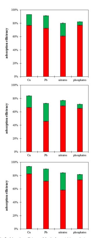
Fig. 3 Adsorption efficiency of lignite for metal ions, nitrates, and phosphates (real water samples): water sampled in June 2023 (a), August 2023 (b), and September 2023 (c). Data are represented as bars, divided into mobile (leachable) fraction (green) and strongly bound (immobilized) fraction (red).
