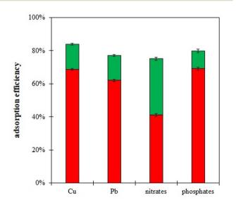
Fig. 2 Adsorption efficiency of lignite for metal ions, nitrates, and phosphates (model solutions). Data are represented as bars, divided into mobile (leachable) fraction (green) and strongly bound (immobilized) fraction (red).
