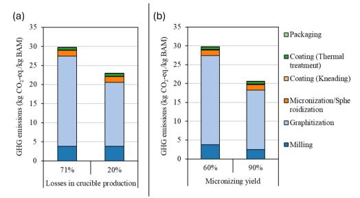
Fig. 6 Greenhouse gas emissions comparison for producing synthetic graphite BAM when varying: (a) the losses in the graphite crucible production, (b) the micronization yield of graphitized powder.
