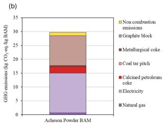
Fig. 3 Greenhouse gas emissions breakdown of synthetic graphite BAM production: (a) per process stage, (b) per input/output flow.
