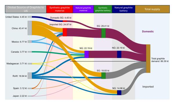
Fig. 9 Graphite supply chain contribution for U.S. EV batteries (NG refers to natural graphite and SG refers to synthetic graphite).
