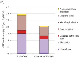
Fig. 11 Impact of switching graphitization and micronization/spheroidization processing steps on greenhouse gas emissions of SG BAM production (a) per process stage, (b) per input/output flow.
