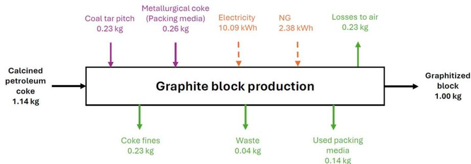
Fig. 2 Process flow diagram of graphite block production.
