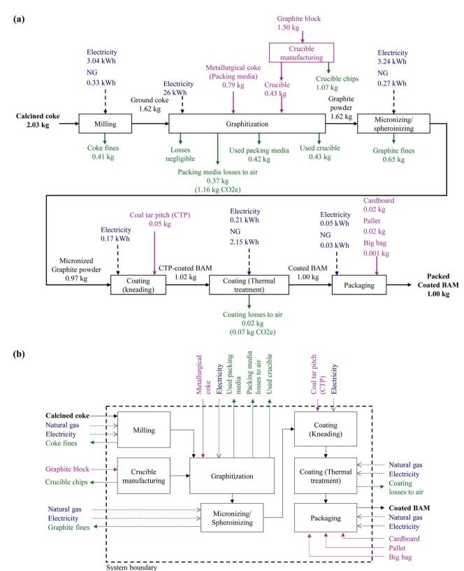
Fig. 1 (a) Process flow diagram of SG BAM production, with values adapted Carrère et al.<sup>28</sup> (refer to Table S3 in the SI for details). (b) System boundary used for the analysis of GHG emissions and fossil energy and water consumption. The blue, magenta, and green fonts indicate energy sources, material sources, and material outputs, respectively.
