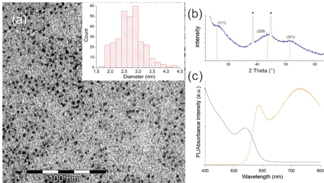
**Fig. 3** (a) TEM image and size distribution of InP QDs ( $\sim 2.7$  nm); (b) XRD pattern showing the zinc blende crystal structure; (c) UV-Vis absorption and PL spectra highlighting band-edge emission ( $\sim 590$  nm) and surface trap emission ( $\sim 710$  nm). Reproduced with permission from ref. 105, copyright 2023 American Chemical Society.
