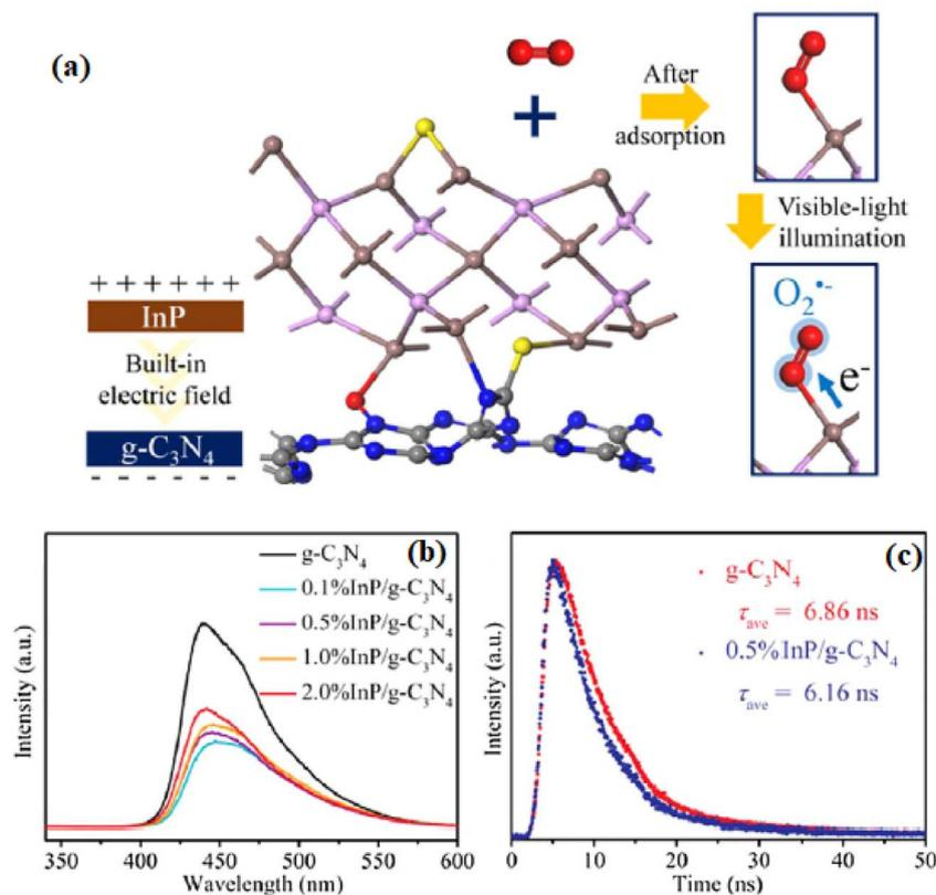
Fig. 6 (a) Schematic of O<sub>2</sub> activation via charge transfer in InP/g-C<sub>3</sub>N<sub>4</sub> under visible light. (b) PL spectra show reduced recombination with InP loading. (c) Time-resolved PL confirms shorter carrier lifetime and improved charge separation. Reproduced from Cao *et al.*, *Chin. Chem. Lett.*, 2020, 31, 2689–2692, under the Creative Commons CC BY license.<sup>172</sup>
