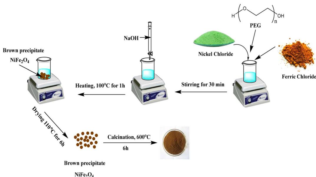
Scheme 1 Schematic representation the preparation of  $\text{NiFe}_2\text{O}_4$  nanoparticles.
