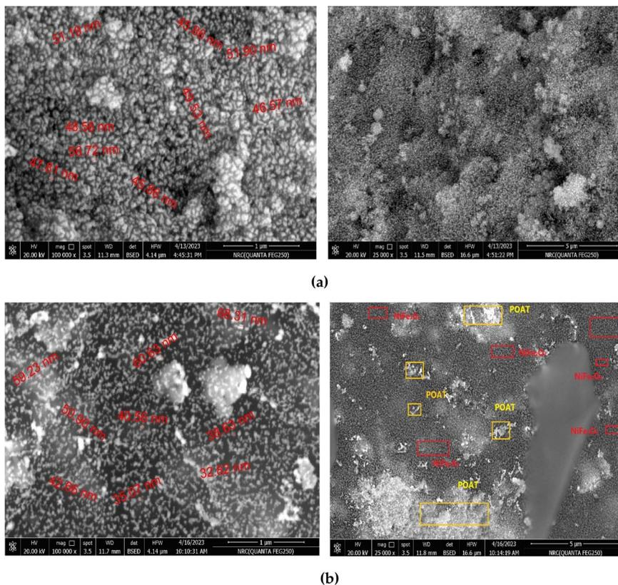
Fig. 2 SEM images of (a) NiFe<sub>2</sub>O<sub>4</sub>, and (b) NiFe<sub>2</sub>O<sub>4</sub> coated with poly[co-*o*-toluidine + aniline].
