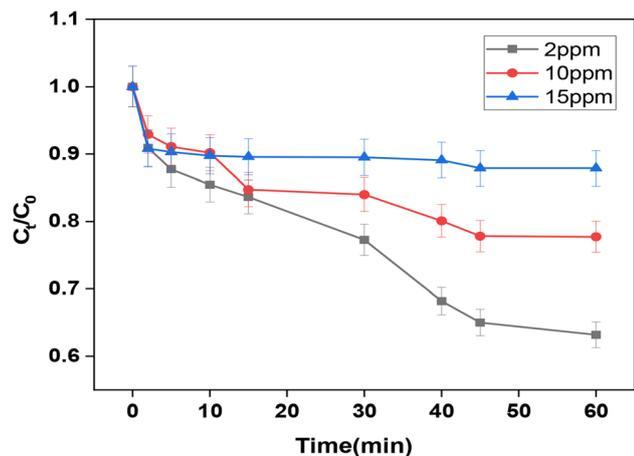
Fig. 7 Effect of  $C_{\text{NiFe}_2\text{O}_4/\text{PAOT}}$  on the reduction of (4-NP) [ $V_{\text{solution}} = 10$  mL,  $T = 25$  °C,  $\text{pH} = 7.43$ ,  $[4\text{-NP}] = 2, 10, 15$  ppm;  $m = 10$  mg].
