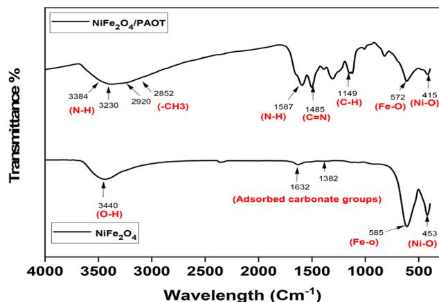
Fig. 1 FTIR spectra of NiFe<sub>2</sub>O<sub>4</sub> nanoparticles and NiFe<sub>2</sub>O<sub>4</sub>/PAOT nanocomposite.
