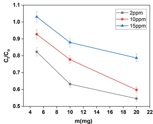
Fig. 10 Effect of dose ( $\text{NiFe}_2\text{O}_4/\text{PAOT}$ ) on the reduction of (4-NP):  $V_{\text{solution}} = 10 \text{ mL}$ ,  $T = 25 \text{ }^\circ\text{C}$ ,  $\text{pH} = 7.43$ ,  $[\text{4-NP}] = 2, 10, 15 \text{ ppm}$ ,  $m = (5, 10, 20) \text{ mg}$ .
