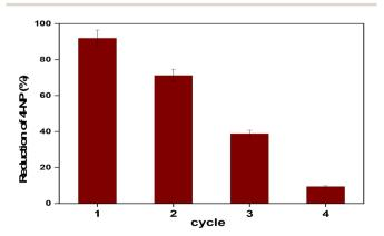
Fig. 13 Reusability of the NiFe<sub>2</sub>O<sub>4</sub>/POAT catalyst for 4-NP reduction.
