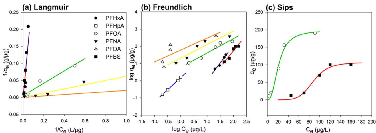
Fig. 4 The adsorption isotherm for PFAS by ABR fitting *via* (a) Langmuir, (b) Freundlich, and (c) Sips isotherm model based on equilibrium concentrations derived dosages ranging from 0.1 to 10 g L<sup>-1</sup>.
