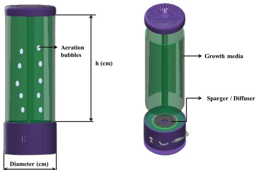
Fig. 1 Design of a photobioreactor.
