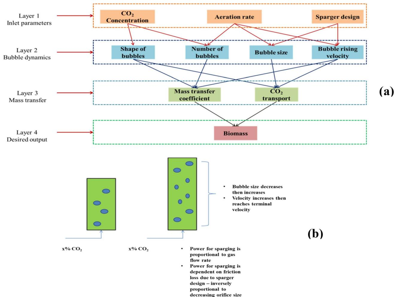
Fig. 7 (a) Photobioreactor design layer by layer approach; (b) size comparison of bubbles according to PBR height.
