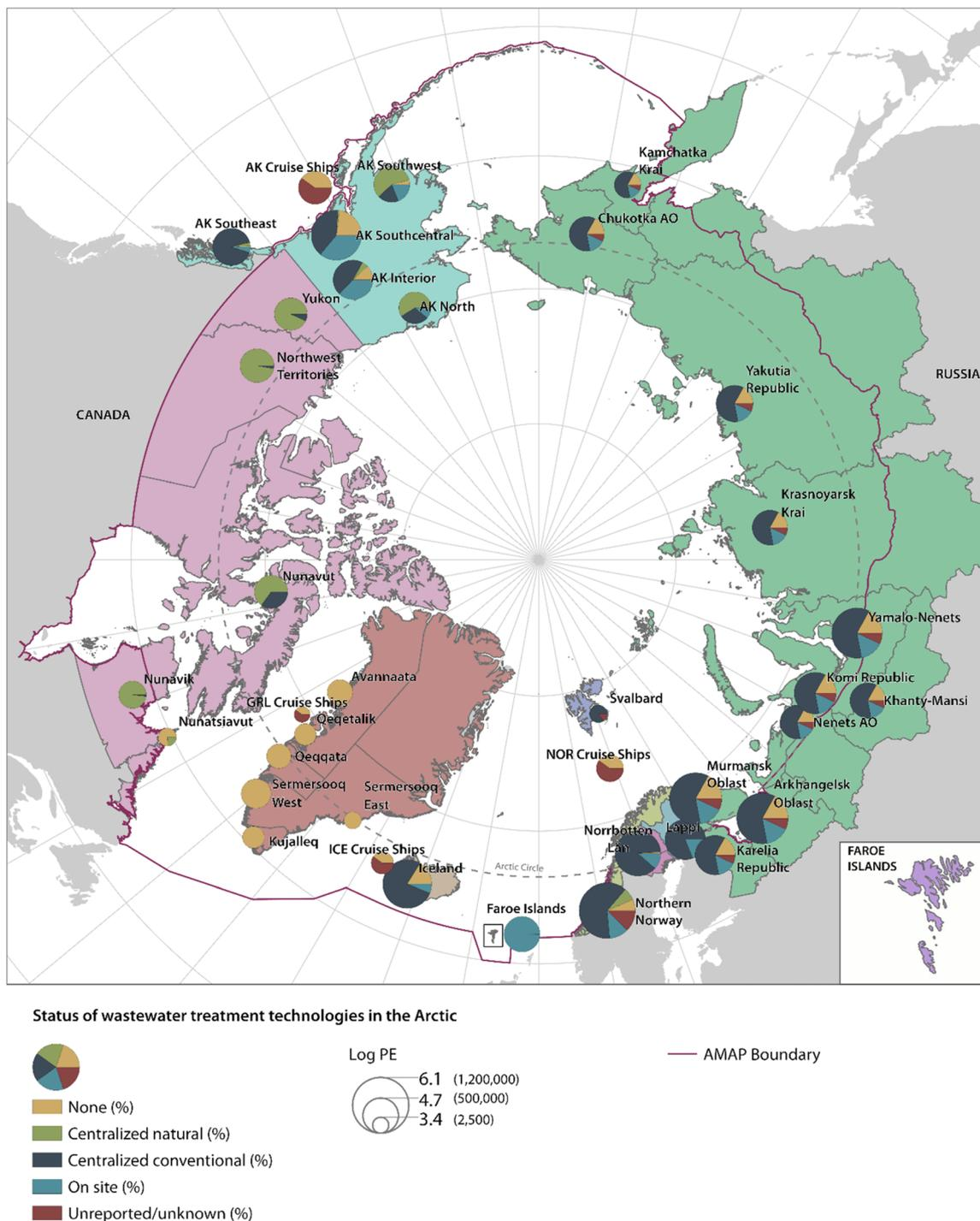
Fig. 1 Wastewater treatment technologies applied and PE load for domestic wastewater in the Arctic region. Centralized natural treatment includes ponds, lagoons, wetlands, and infiltration systems; conventional plants include systems ranging from preliminary screening to advanced/tertiary; on-site treatment includes septic tanks with/without drainfield, small infiltration systems and package plants as well as outhouses.
