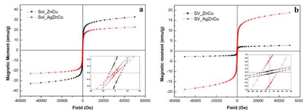
Fig. 5 Magnetic measurements of  $\text{Zn}_{0.5}\text{Cu}_{0.5}\text{Fe}_2\text{O}_4$  and  $\text{Zn}_{0.5}\text{Cu}_{0.5}\text{Fe}_2\text{O}_4$  functionalized with silver. (a) Sol-gel synthesized nanomaterials (Sol\_ZnCu and Sol\_AgZnCu); (b) solvothermal synthesized nanomaterials (SV\_ZnCu and SV\_AgZnCu).
