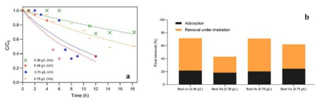
Fig. 10 Assays using the best conditions for different photocatalyst concentration of (a)  $0.36 \text{ g L}^{-1}$  and (b)  $0.75 \text{ g L}^{-1}$ ; (c) final removal of the performed assays using the best conditions.
