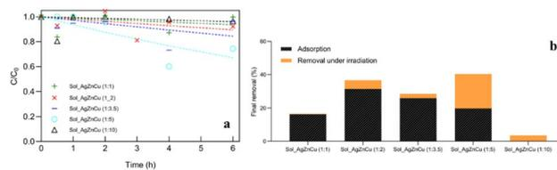
Fig. 8 Activity of  $\text{Zn}_{0.5}\text{Cu}_{0.5}\text{Fe}_2\text{O}_4$  synthesized by sol-gel and functionalized with different amounts of silver: (a) adsorption assays with visible light irradiation assays with  $\text{Sol\_AgZnCu}$ ; (b) final removal.
