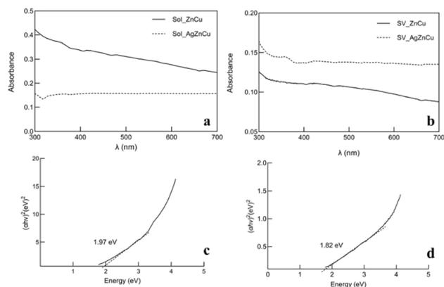
Fig. 3 UV-vis absorption spectra of  $Zn_{0.5}Cu_{0.5}Fe_2O_4$  nanomaterials ( $1 \text{ g L}^{-1}$ ): (a) synthesized by sol-gel and Ag-doped; (b) solvothermal synthesized  $Zn_{0.5}Cu_{0.5}Fe_2O_4$  functionalized with Ag; (c) Tauc plot for  $Zn_{0.5}Cu_{0.5}Fe_2O_4$  by sol-gel method; (d) Tauc plot for  $Zn_{0.5}Cu_{0.5}Fe_2O_4$  by solvothermal method.
