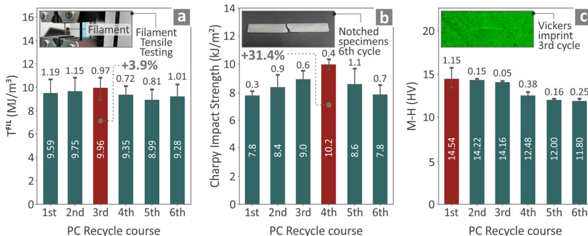
Fig. 6 Results from the samples tested from every recycling cycle of the PC. (a) Filament toughness  $T^{FIL}$ , (b) impact strength (Charpy), and (c) M-H measurements on samples, all accompanied by images captured during the testing procedures.
