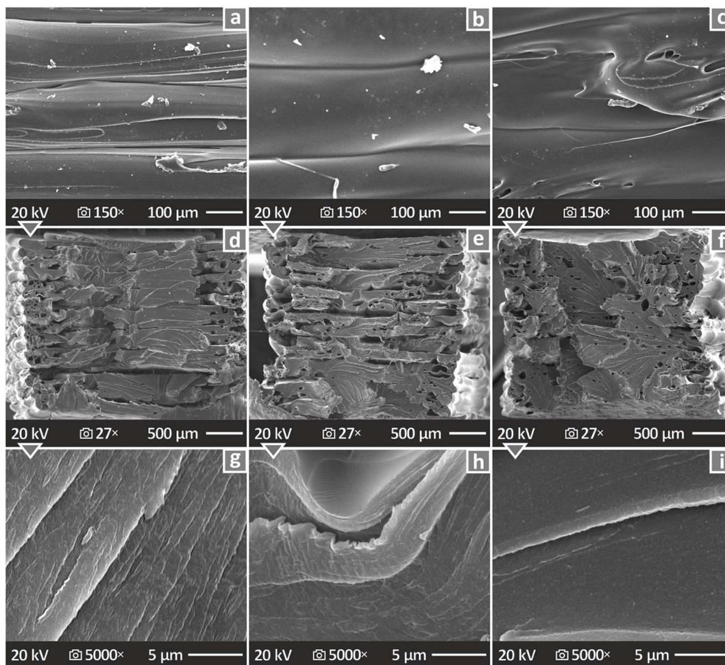
Fig. 10 (a–c) SEM images of 150 $\times$  magnification demonstrating the vertical surface of the PC first, third, and sixth samples, (d–f) SEM images of 27 $\times$  and (g–i) SEM images of 1000 $\times$  magnification demonstrating the fracture surface of the PC first, third, and sixth cycle samples.
