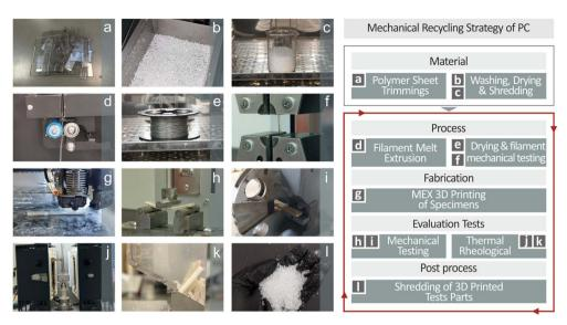
Fig. 1 The steps followed in this research and the mechanical recycling strategy for the PC polymer. On the right side, the flow diagram of the process is depicted, and on the left side, corresponding screenshots for each step are shown.
