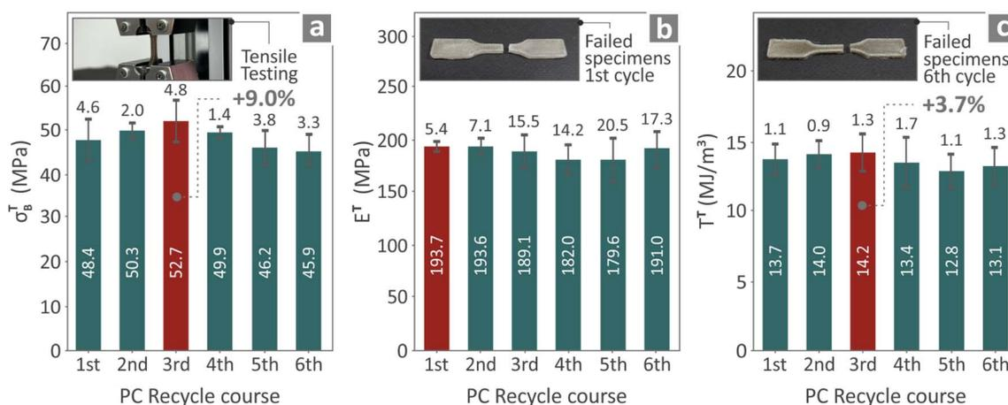
Fig. 4 The tensile properties of the samples from the six PC recycling courses are presented. In detail, (a)  $\sigma_b^T$  results accompanied by an image during the testing, (b)  $E^T$  results accompanied by an image of the tested specimens of the first cycle and (c)  $T^T$  results accompanied by an image of the tested specimens of the sixth cycle.
