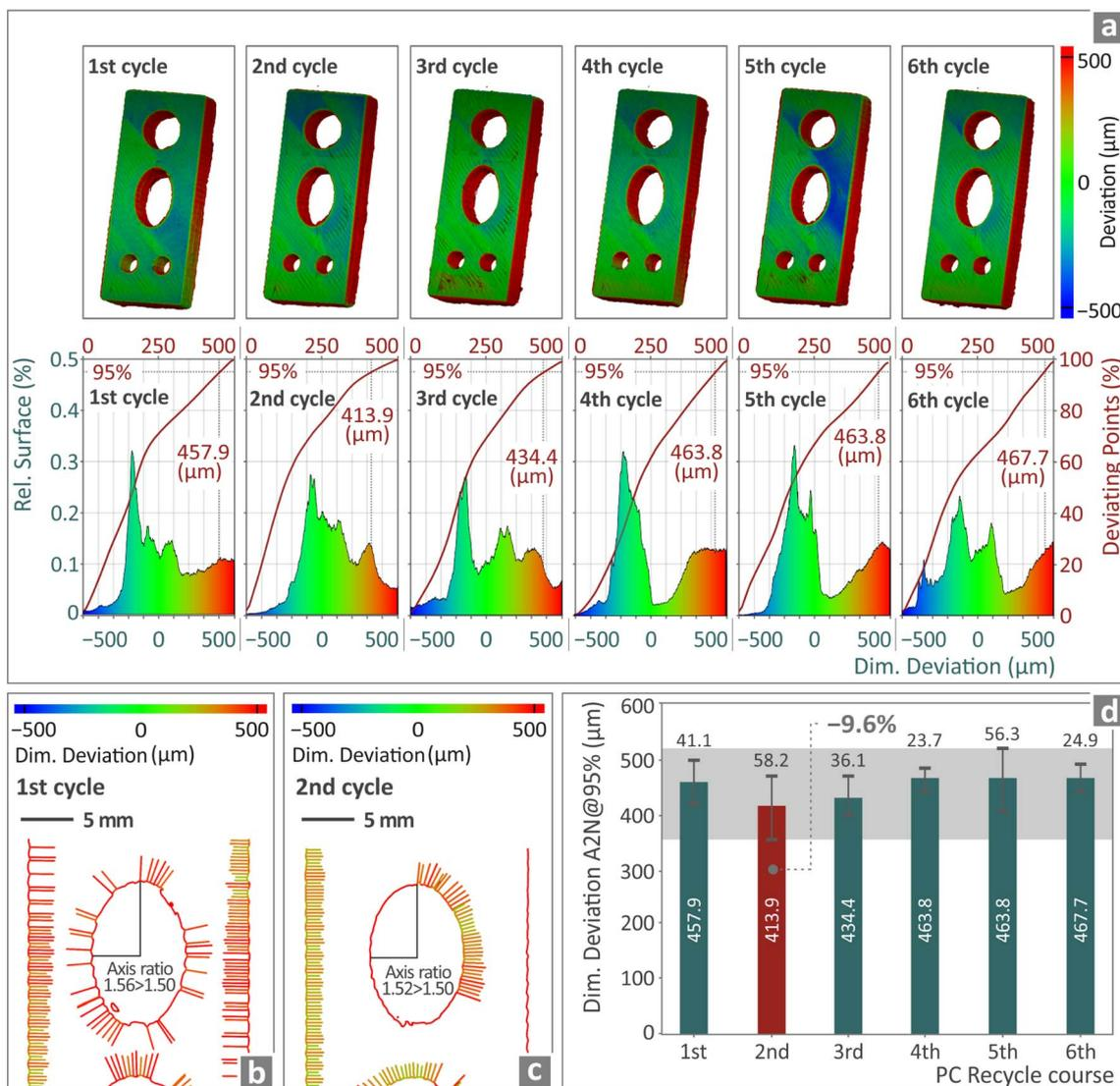
Fig. 12 (a) Color-coded mapping of the samples' dimensional deviation for each recycling cycle, including associated surface and deviating point graphs vs. dimensional deviation. (b and c) A color-coded mapping representation of sections from the first and second PC recycling cycles' dimensional deviation and (d) the levels of all PC recycling cycles' dimensional deviation.
