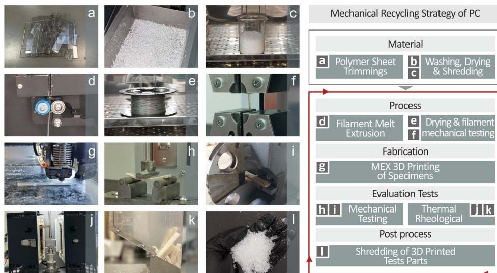
Fig. 1 The steps followed in this research and the mechanical recycling strategy for the PC polymer. On the right side, the flow diagram of the process is depicted, and on the left side, corresponding screenshots for each step are shown.
