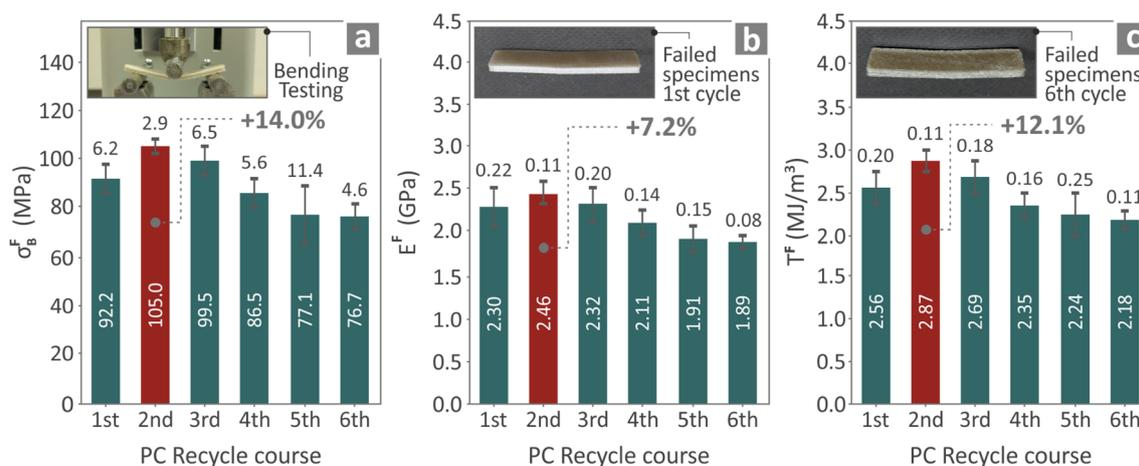
Fig. 5 The flexural properties of the tested flexural specimens from the six PC recycling cycles are presented namely (a) the  $\sigma_b^F$  (flexural strength) outcome accompanied by an image from the testing, (b)  $E^F$  (flexural modulus) outcome and image from the first course's tested specimens, and (c)  $T^F$  (flexural toughness) outcome accompanied by an image from the tested specimens of the sixth cycle.
