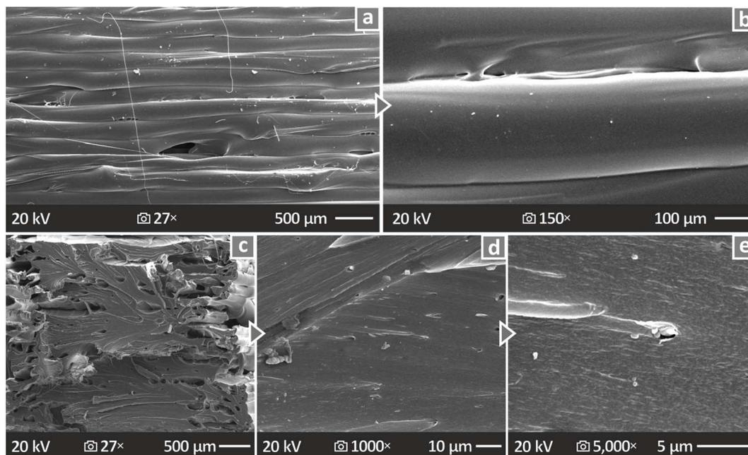
Fig. 11 (a and b) SEM image of 27 $\times$  magnification demonstrating the side surface of the PC second recycling cycle and 150 $\times$  magnification, (c–e) demonstrating an image of the fractured surface, in 27 $\times$ , 1000 $\times$  and 5000 $\times$  magnification, of the PC second recycling cycle.
