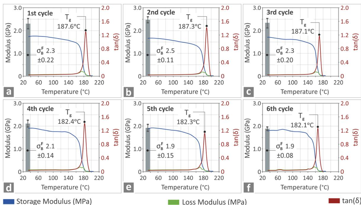
Fig. 3 DMA results in graphs of flexural modulus, loss and storage modulus,  $\tan(\delta)$  versus temperature modulus for every one of the six recycling cycles of PC. (a) 1st cycle, (b) 2nd cycle, (c) 3rd cycle, (d) 4th cycle, (e) 5th cycle, (f) 6th cycle.
