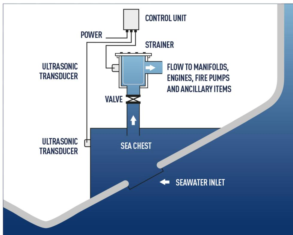
Fig. 4 Recommended ultrasonic anti-fouling system.<sup>55</sup>
