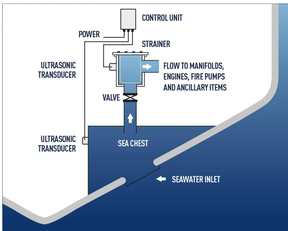
Fig. 4 Recommended ultrasonic anti-fouling system.<sup>55</sup>
