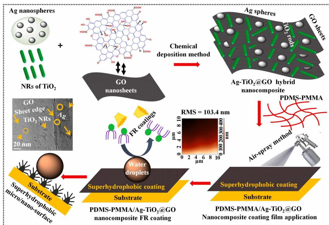
Fig. 5 Preparation stages of a PDMS-PMMA/Ag-TiO<sub>2</sub>-GrO hybrid nanocomposite *via* the solution-casting method as a superhydrophobic and FR coating.<sup>66</sup>
