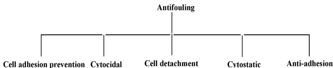
Fig. 2 Classification of anti-fouling materials.
