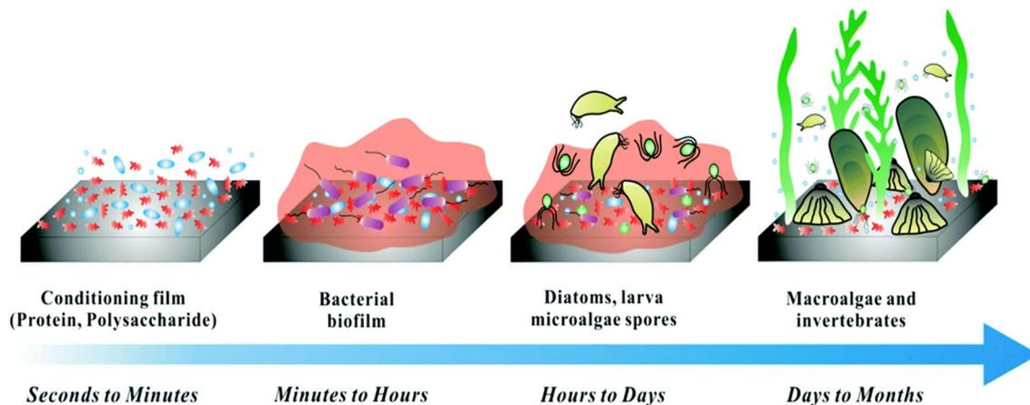
Fig. 1 The steps in the process of bio-fouling.<sup>1</sup>
