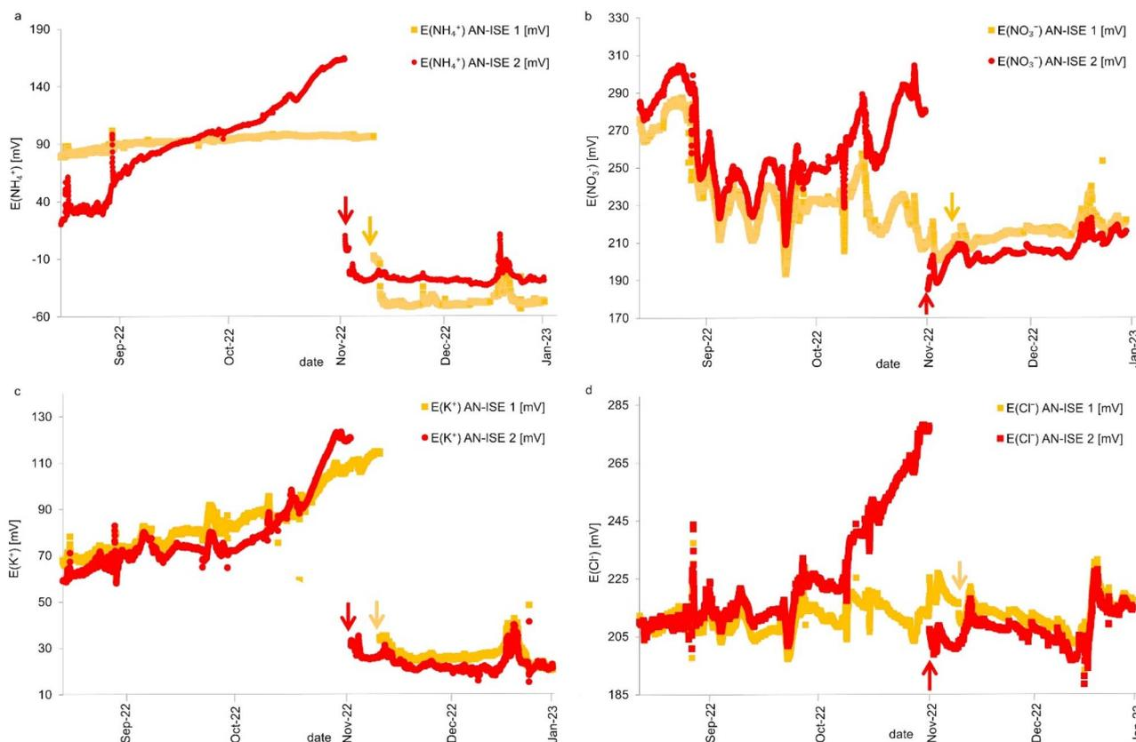
Fig. 6 Drift of mV signals: mV signals from AN-ISE 1 and 2 for (a)  $\text{NH}_4^+$ , (b)  $\text{NO}_3^-$ , (c)  $\text{K}^+$  and (d)  $\text{Cl}^-$  over the entire measurement period (arrows: cartridge replacement).
