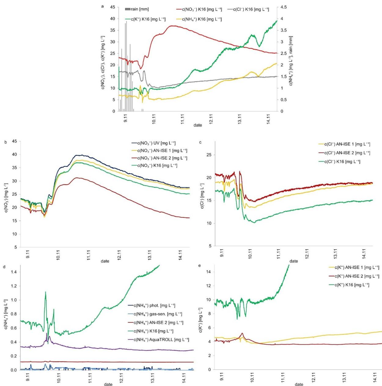
Fig. 5 Event vs. drift: (a)  $\text{NH}_4^+$ ,  $\text{NO}_3^-$ ,  $\text{K}^+$  and  $\text{Cl}^-$  readings of K16 ISE, (b)  $\text{NO}_3^-$  readings of UV probe and AN-ISE 1, AN-ISE 2 and K16 ISEs, (c)  $\text{Cl}^-$  readings of AN-ISE 1, AN-ISE 2 and K16 ISEs, (d)  $\text{NH}_4^+$  readings of photometric and gas-sensitive analysers and AN-ISE 2, K16 and AquaTROLL ISEs, (e)  $\text{K}^+$  readings of AN-ISE 1, AN-ISE 2 and K16 ISEs; Bickenalb River, 09–14.11.2022.
