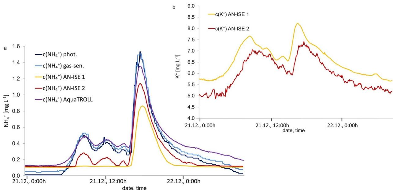
Fig. 3 (a) Event detection:  $\text{NH}_4^+$  readings from the photometric and gas-sensitive analysers, AN-ISE 1 and AN-ISE 2 (with ion interference compensation) and AquaTROLL (without compensation), (b)  $\text{K}^+$  readings from AN-ISE 1 and 2; Bickenalb River, 21.–22.12.2022.
