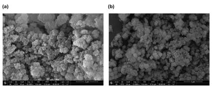
Fig. 4 FESEM images of poly(AN-co-AMPS) with different scales: 3 μm (a) and 5 μm (b).
