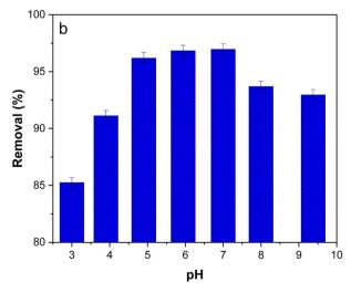
PCZ of poly(AN-co-AMPS) (a) and effect of pH on the adsorption of BG onto poly(AN-co-AMPS) (b).
