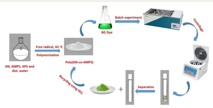
Fig. 1 Experimental design of the removal of hazardous BG dve using poly(AC-co-AMPS)
