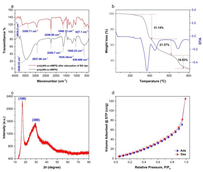
Fig. 3 FTIR spectra of poly(AN-co-AMPS) before and after adsorption (a); TGA analysis of poly(AN-co-AMPS) (b); XRD pattern of poly(AN-co-AMPS) (c); and N<sub>2</sub> adsorption-desorption isotherm of poly(AN-co-AMPS) (d).
