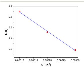
Fig. 10 Plot of  $\ln K_c$  against 1/T for BG dye adsorption onto poly(ANco-AMPS).
