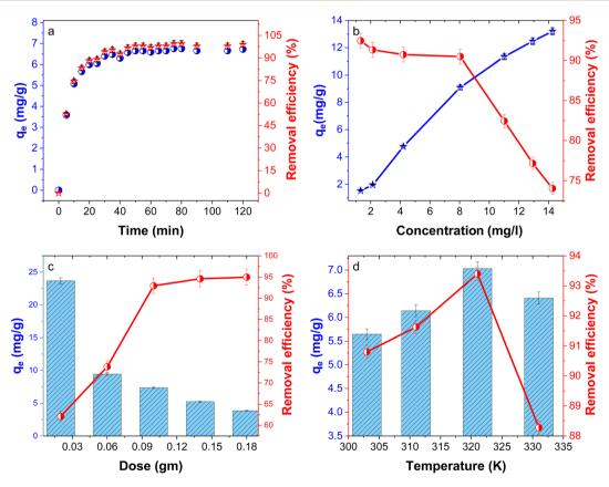
Fig. 6 Effect of contact time on the adsorption of BG onto poly(AN-co-AMPS) (a); effect of initial concentration of BG on adsorption process (b); effect of poly(AN-co-AMPS) dose on the adsorption of BG dye (c); and effect of temperature on BG adsorption onto poly(AN-co-AMPS) (d).
