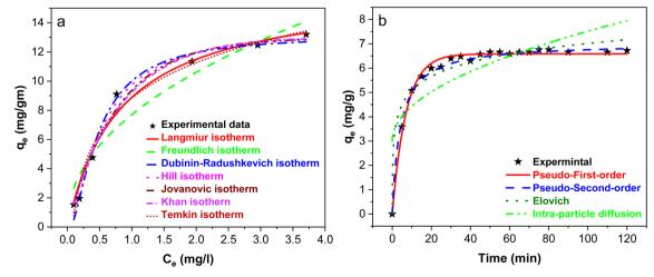
Fig. 9 Adsorption isotherms of BG onto poly(AN-co-AMPS) (a) and adsorption kinetic models of BG onto poly(AN-co-AMPS) (b).
