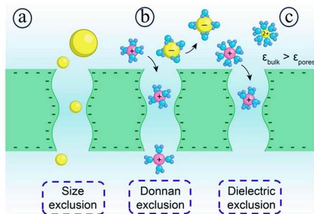
Fig. 2 Three primary membrane separation mechanisms: (a) size exclusion, (b) Donnan exclusion, and (c) dielectric exclusion (reprinted with permission from ref. 21, Wiley 2023).
