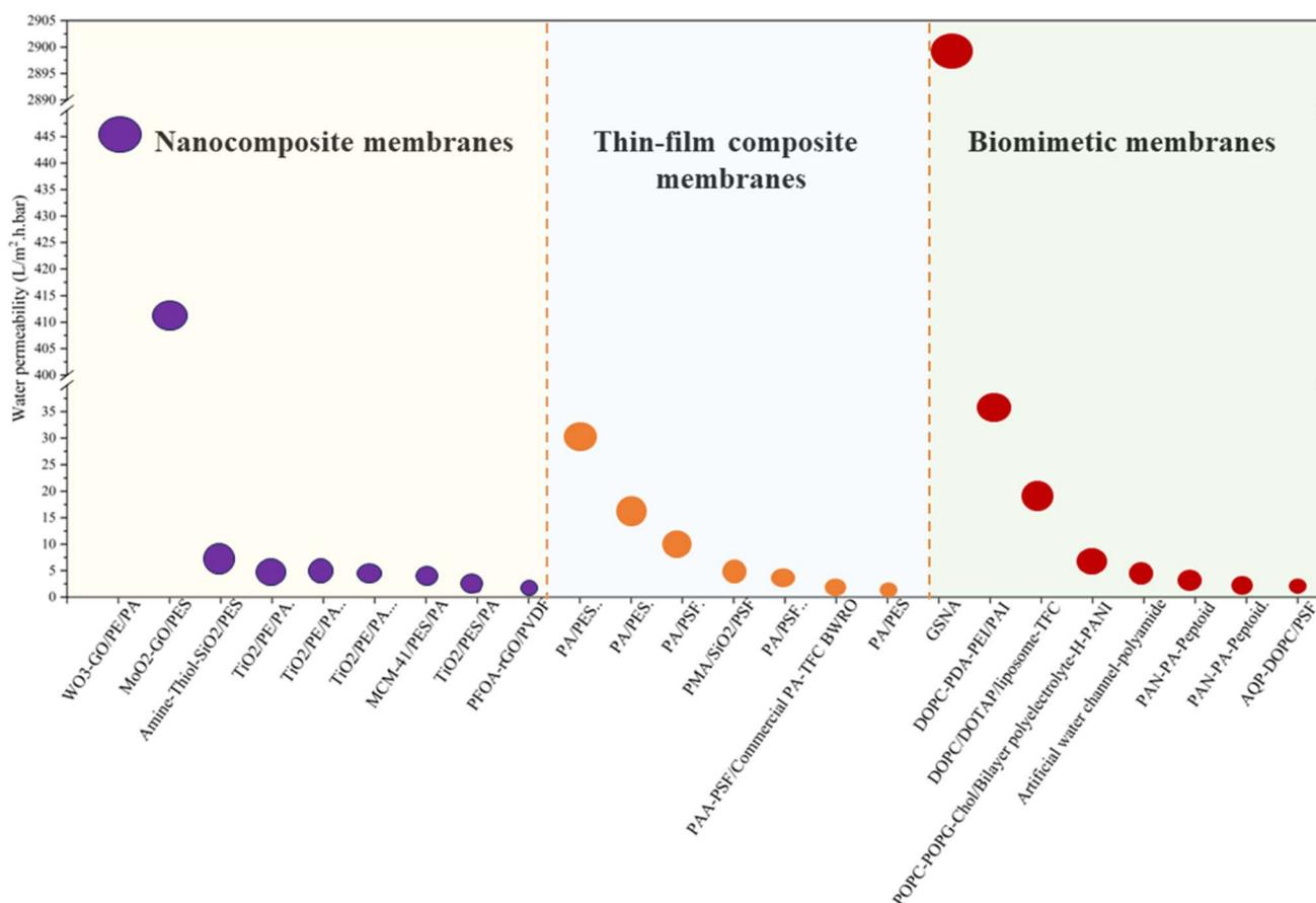
Fig. 10 Permeability of the selected membranes obtained through literature survey and screening in the present study.
