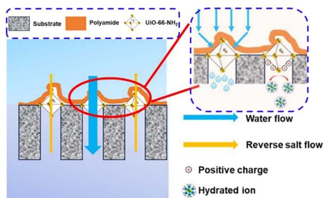
Fig. 9 PA/Zr-MOF (UiO-66-NH<sub>2</sub>)/ceramic-based FO membrane (reprinted with permission from ref. 280, Elsevier 2024).
