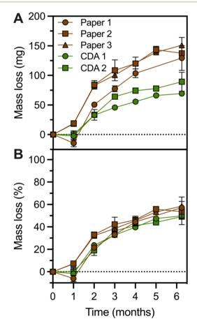
Fig. 2 (A) Absolute mass loss (in mg) and (B) relative mass loss (%) of the paper (brown) and CDA (green) CFs in the flow-through mesocosm throughout the six-month experiment. Data are presented as the mean  $\pm$  standard deviation. In some cases, error bars are smaller than the symbol. Values and replication are presented in Tables S2 and S3.†
