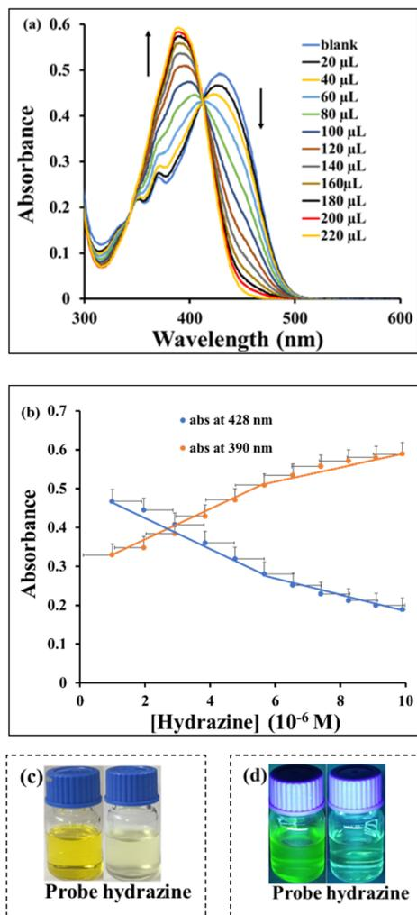
Fig. 1 (a) Overlaid absorption spectra of probe 1 ( $10^{-5}$  M) with hydrazine ( $10^{-4}$  M) in THF, (b) absorbance at 390 nm and 428 nm with increasing concentration of hydrazine. Colour changes of the probe with hydrazine visible with (c) naked eye and (d) under a UV lamp.
