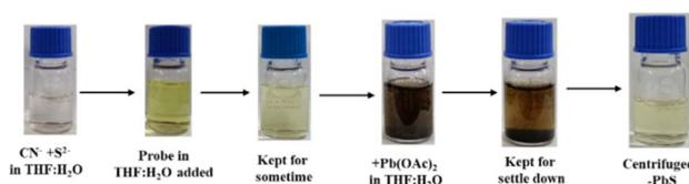
Fig. 4 Experiment performed for selective sensing of  $\text{CN}^-$  in the presence of both  $\text{S}^{2-}$  and  $\text{CN}^-$ .  $\text{Pb}(\text{OAc})_2$  was added to the mixture after the addition of the probe to remove  $\text{S}^{2-}$  as  $\text{PbS}$ .
