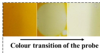
Fig. 7 Colour changes of the probe in the vapor phase upon exposure to 10 mM hydrazine solution.
