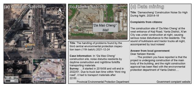
Fig. 2 Verification of construction site: an example for monitoring station 1201C. Process: (a) locate a potential construction site around 1201C using Google Satellite. (b) Access the construction's name using Baidu Satellite. (c) Conduct data mining on the internet. In this case, construction was active during the target period with overnight construction activities, leading to many complaints from nearby residents.
