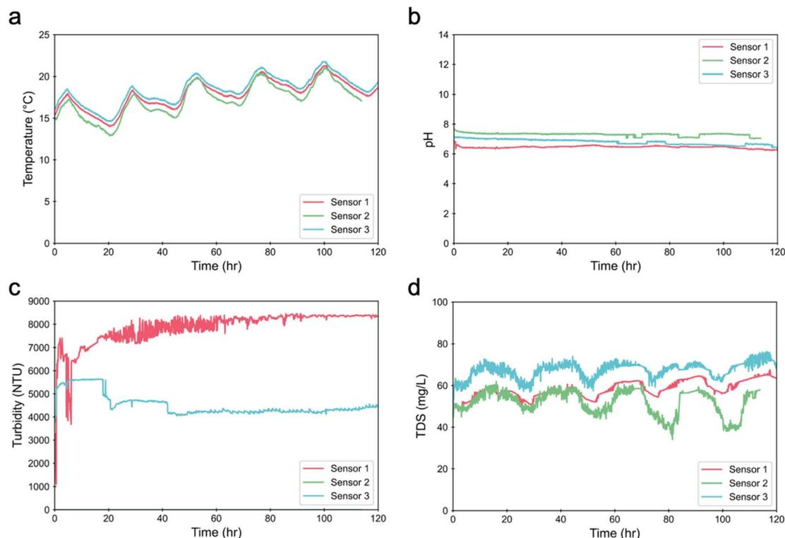
Fig. 4 Precision assessment of the low-cost water quality sensor system using three identical units deployed under similar environmental conditions. (a) Temperature, (b) pH, (c) turbidity, and (d) total dissolved solids (TDS) measurements from each unit are represented by different colored lines.
