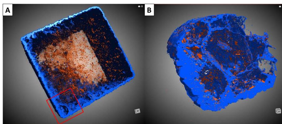
Fig. 4 Synchrotron tomography rendering of the marble sample Carrara-04 reacted for 16 days in a 2 M CdCl<sub>2</sub> solution. The replaced phase appears in blue and the porosity is in red. (A) Full cube with a voxel size of 2.3 μm and (B) a corner of the same sample with a voxel size of 0.36 μm showing both the external reaction rim and some reaction product along grain boundaries. From these data, the reacted volume is calculated.
