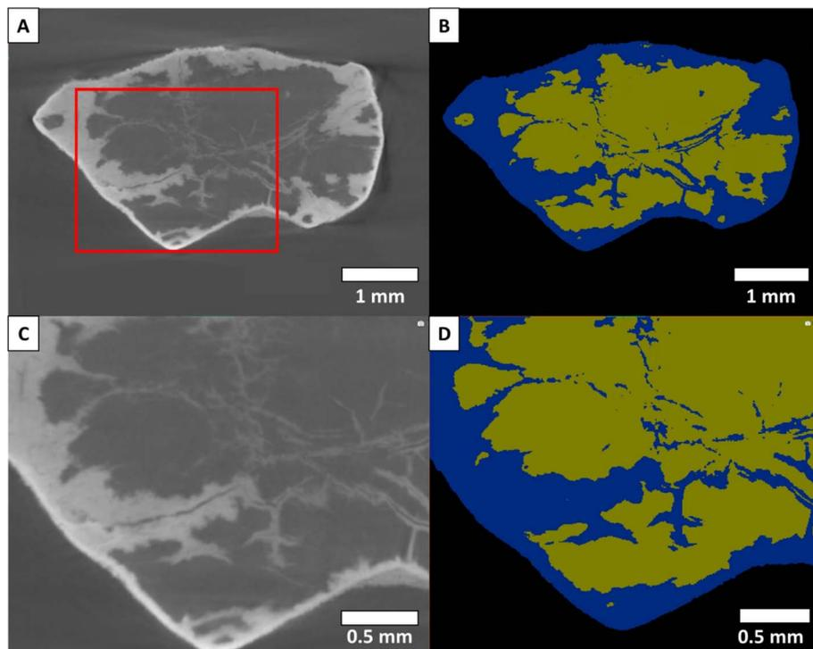
Fig. 2 X-ray tomography imaging of sample Aragonite-04 reacted for 16 days in 2 M CdCl<sub>2</sub>: (A) original X-ray tomography slice, (B) after segmentation (yellow: aragonite, blue: solid solution of (Ca,Cd)CO<sub>3</sub>, black: background). (C and D) are zooms into respectively (A and B), the zoom area is indicated by the red area in A. The transformation of aragonite into a solid solution that contains cadmium occurred by a process of reaction-induced fracturing.
