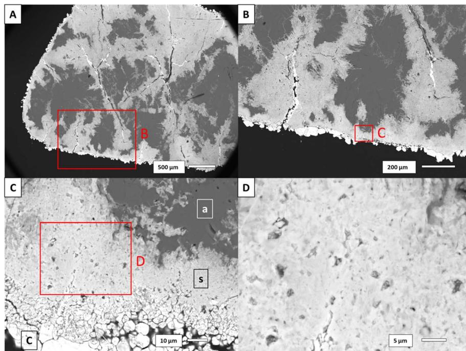
Fig. 5 Back-scattered electron images of sample Aragonite-03 reacted for 64 days in a 0.4 M  $\text{CdCl}_2$  solution with (A) the full sample and (B–D) are consecutive zooms in the areas indicated in red in the previous images. The labels in C indicate the different phases are: (a) aragonite, (s) the  $(\text{Ca,Cd})\text{CO}_3$  solid solution and (c) the  $\text{CdCl}_2$  crystals.
