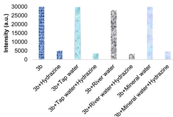
Fig. 7 Emission intensity of SBC **3b** (0.5  $\mu\text{M}$ ; 537 nm) after the addition of different water samples in methanol with and without hydrazine.
