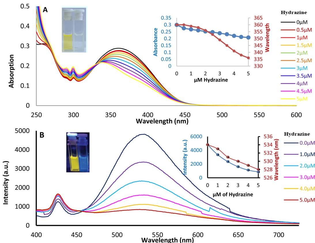
Fig. 3 Hydrazine (0.0 to 5.0  $\mu\text{M}$ ) vs. SBC **3b** (5.0  $\mu\text{M}$ ) titration by (A) UV-vis absorption and (B) fluorescence emission ( $\lambda_{\text{ex}} = 358 \text{ nm}$ ) studies in methanol.
