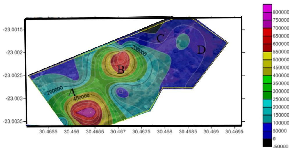
Fig. 7 Spatial variation of CH<sub>4</sub> emissions from the landfill determined using Surfer software.
