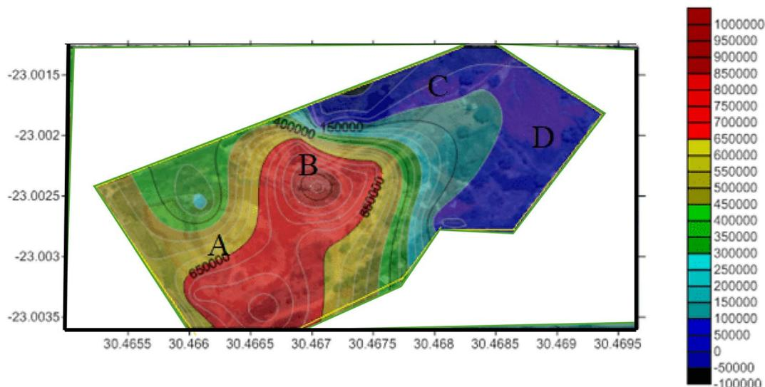
Fig. 8 Spatial variation of CO<sub>2</sub> emissions from the landfill determined using Surfer software.
