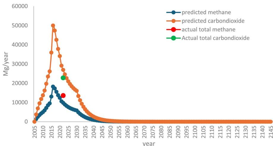
Fig. 10 The annual average CH<sub>4</sub> and CO<sub>2</sub> measured and estimated from the landfill.
