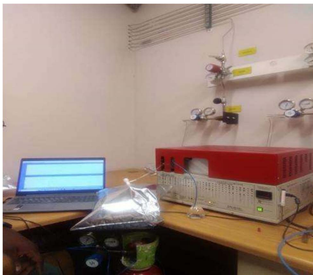
Fig. 5 The analysis of the gases collected from the Thohoyandou landfill site.
