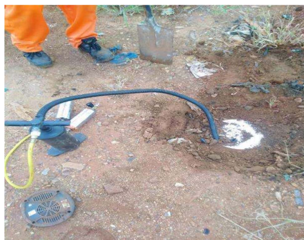
Fig. 3 The collection of gases using the flux chamber and a handheld pump.
