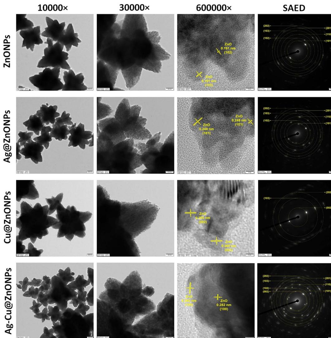
Fig. 7 HR-TEM images showing the lattice and SAED pattern of the undoped and doped ZnONPs.
