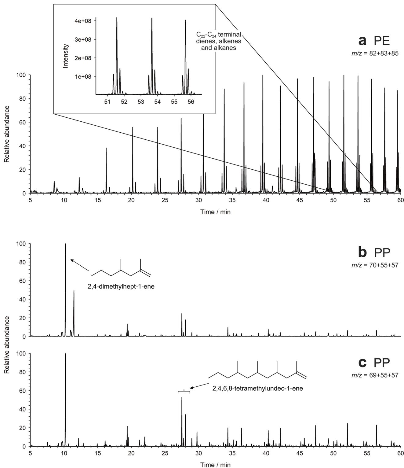
Fig. 3 Partial Py-GC-MS chromatograms of (a) sand spiked with PE, extracted using density separation *via* overnight settling, filtered by  $m/z$  82 + 83 + 85, and (b) and (c) soil spiked with PP, extracted using density separation *via* overnight settling and hydrogen peroxide digestion in a beaker, filtered by (b)  $m/z$  70 + 55 + 57 and (c)  $m/z$  69 + 55 + 57.
