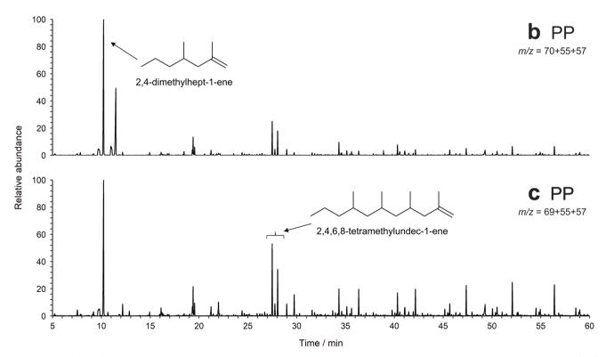
Fig. 3 Partial Py-GC-MS chromatograms of (a) sand spiked with PE, extracted using density separation via overnight settling, filtered by m/z 82 + 83 + 85, and (b) and (c) soil spiked with PP, extracted using density separation via overnight settling and hydrogen peroxide digestion in a beaker, filtered by (b) m/z 70 + 55 + 57 and (c) m/z 69 + 55 + 57.
