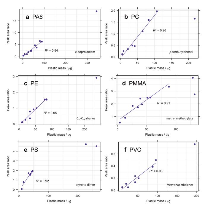
Fig. 2 Calibration curves for (a) PA6, (b) PC, (c) PE, (d) PMMA, (e) PS and (f) PVC created from the ion chromatogram peak area ratio of each selected diagnostic compound with anthracene- $d_{10}$  or pyrene- $d_{10}$  as the internal standard, with additional standards outside the calibration range added.
