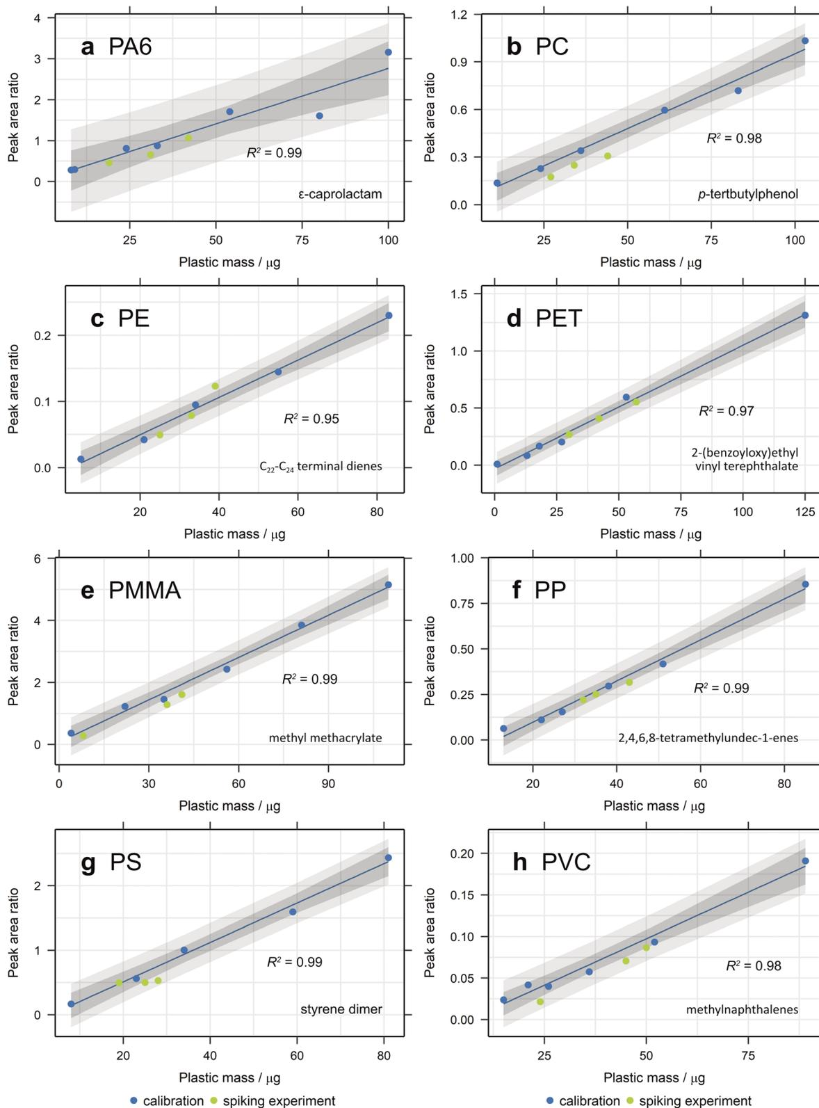
Fig. 4 Recovery of (a) PA6, (b) PC, (c) PE, (d) PET, (e) PMMA, (f) PP, (g) PS and (h) PVC from spiked samples after density separation *via* overnight settling and hydrogen peroxide digestion in a beaker. Calibration curves were created from the ion chromatogram peak area ratio of each selected diagnostic compound with anthracene- $\text{d}_{10}$  or pyrene- $\text{d}_{10}$  as the internal standard and 95% confidence and prediction bands plotted.
