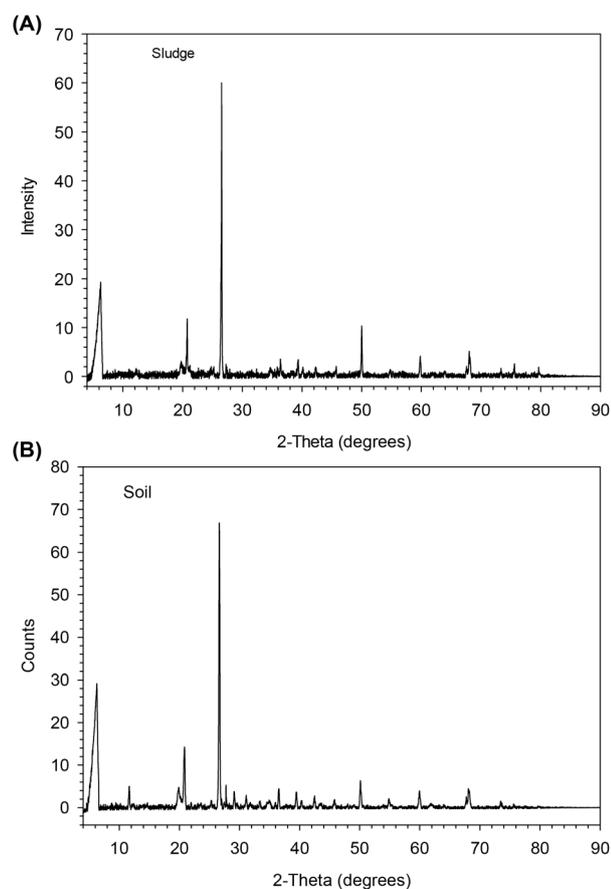
Fig. 4 XRD patterns of (A) sludge and (B) soil. The assignment of peaks in sludge (STC) is given in ref. 11 and 37 with  $d$ -spacing and  $h, k, l$  values. The  $2\theta$  peak values of soil are remarkably similar to those of STC.
