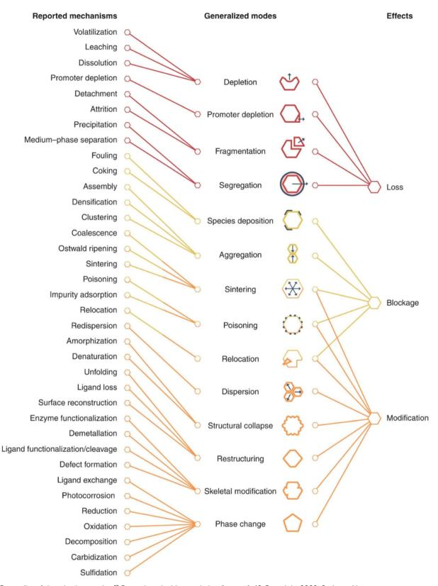
Fig. 5 Generality of deactivation modes.<sup>42</sup> Reproduced with permission from ref. 42 Copyright 2022, Springer Nature.
