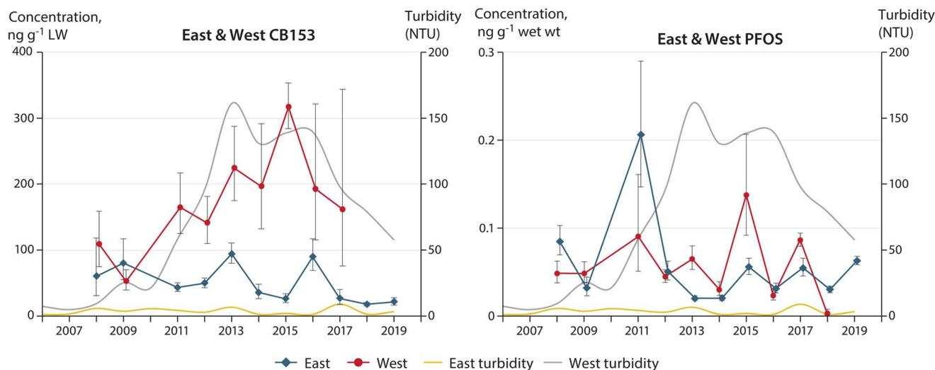
Fig. 11 Long term trends in concentrations of (A) hexachlorobiphenyl PCB153 (ng per g lipid weight (LW)), and (B) perfluorooctane sulfonate (PFOS) (ng per g wet wt) in muscle of landlocked Arctic char from West Lake and East Lake (Melville Island, Canada) (Cabrerizo *et al.*<sup>135</sup> and unpublished data). The trends of turbidity (NTUs) in West and East Lake are also shown.
