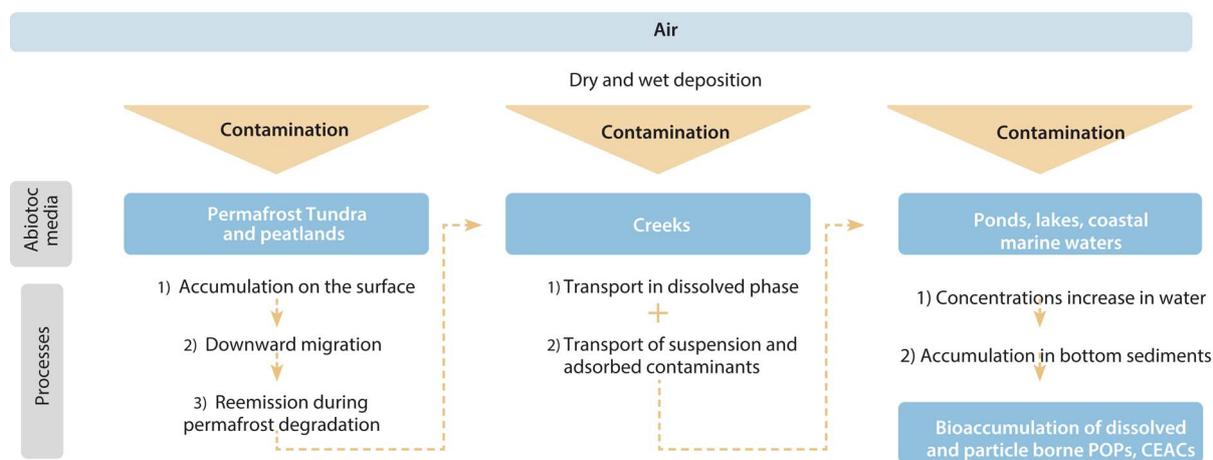
Fig. 6 Environmental fate of organic contaminants delivered to Arctic terrestrial environments *via* long-range atmospheric transport and incorporated into abiotic components. From Potapowicz *et al.*<sup>92</sup>
