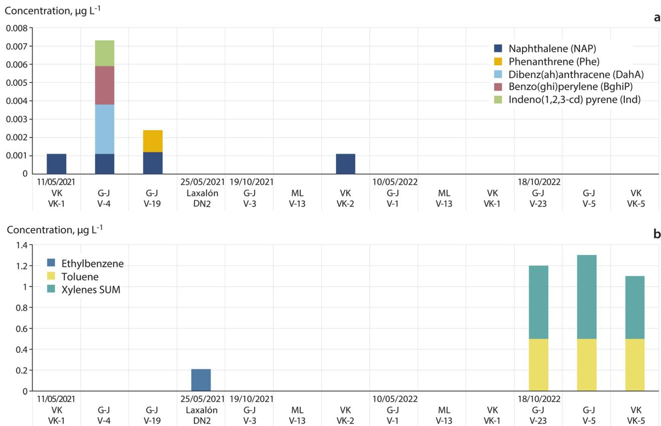
Fig. 16 (a) PAHs detected in samples ( $\mu\text{g L}^{-1}$ ) from four boreholes at two water intake zones after a wildfire incident. (b) BTEX detected in water samples ( $\mu\text{g L}^{-1}$ ) during 2021 and 2022 at multiple sampling times after a wildfire incident (DN = drinking water from the distribution network).<sup>169</sup>
