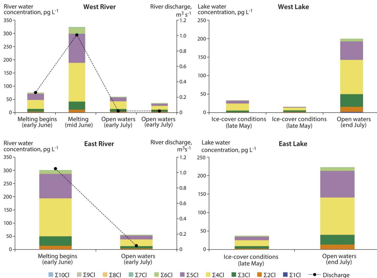
Fig. 10 PCB concentrations (sum of 70 congeners of varying chlorination level,  $Cl_1$  to  $Cl_{10}$ ) in dissolved phase during snowmelt runoff (mid-June) and ice free conditions (mid-July) in West and East Rivers on Melville Island, 2016. Redrawn from Cabrerizo *et al.*<sup>135</sup>
