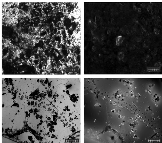
Fig. 5 Visible (left) and fluorescent (right) images of polyethylene terephthalate microplastic fragment from a soil sample (top) and images of a variety of MPs as well as non-labelled minerals and organic matter from sediments sample (bottom). Scale bars are 100 microns.
