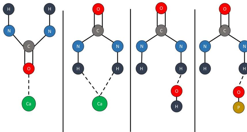
Fig. 4 Proposed bonding modes between Ca<sup>2+</sup>, O<sub>3</sub>–PO<sub>3</sub><sup>3-</sup>, and OH<sup>-</sup> in HAP with –CO, and NH– functional groups of urea.<sup>35</sup> Assignments were made based on previous literature reports using metal–urea complexes.
