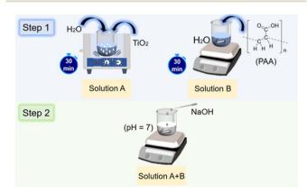
Fig. 1 Diagram illustrating the process of preparing the dip-coating solution for the impregnation of PU foams with TiO2 nanostructures. Steps 1 and 2 illustrate the preparation of solutions A, B and A + B, respectively
