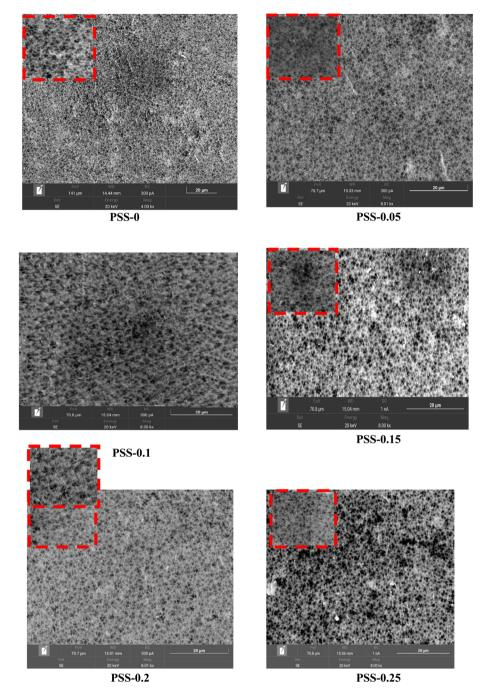
Fig. 8 SEM of the top surface of the pristine membrane and MMMs.
