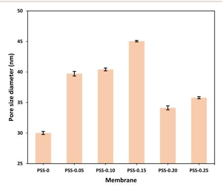
Fig. 11 PVC/SiO<sub>2</sub>-SDS MMMs mean pore size diameter compared with the pristine membrane.
