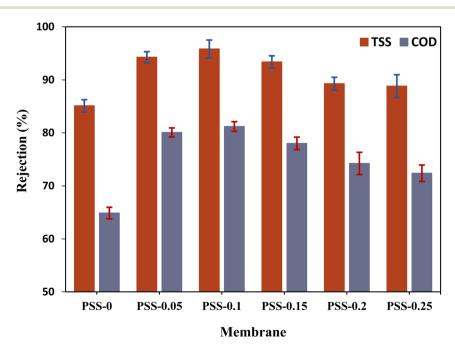
Fig. 13 Rejection% for total suspended solid (TSS) and COD for carwash wastewater by the pristine membrane and MMMs ( $25 \pm 1$  °C, and 1 bar).
