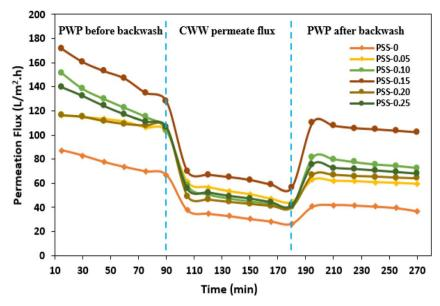
Fig. 14 Time-dependent permeation flux for the pristine membrane and MMMs, as follows: the first 90 min for pure water flux, the second 90 min for flux of carwash wastewater (CWW) and the third for pure water flux after the fouled membranes had undergone one hour of backflushing with pure water.
