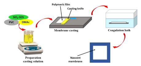
Fig. 2 Preparation of mixed matrix membranes.
