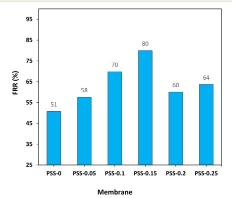
Fig. 15 The flux recovery ratio (FRR) of the pristine membrane and MMMs. The observed changes in the MMMs were found to be statistically significant with a p-value of 0.0178.
