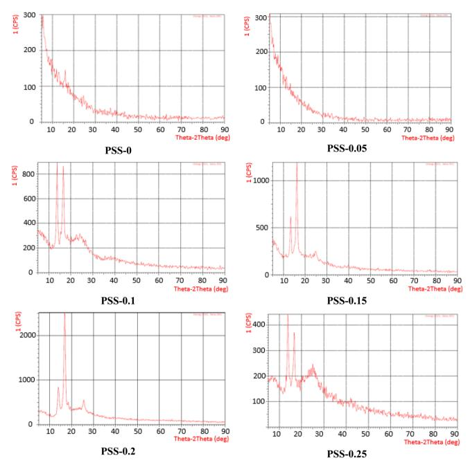
Fig. 5 XRD of the pristine membrane and MMMs.
