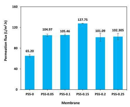
Fig. 12 Pure water flux of a pristine membrane and MMMs prepared with different concentrations of SiO<sub>2</sub>-SDS NPs. The increase in permeate flux of the modified membranes is statistically significant compared to that of the pristine membrane (p-value = 0.0009).
