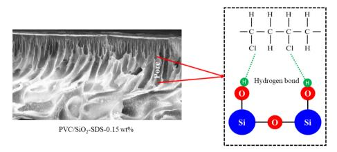
Scheme 2 Antifouling mechanism of the membranes modified by SiO<sub>2</sub>-SDS NPs.
