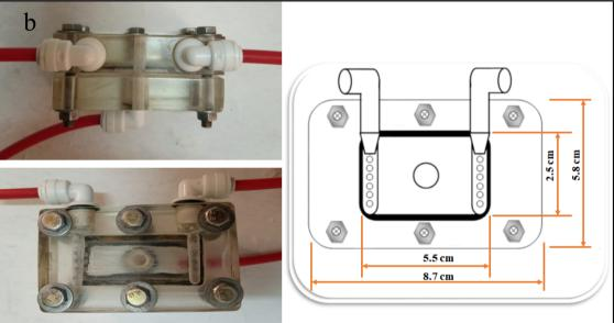
Fig. 3 (a) Schematic diagram of the cross-flow filtration unit. (b) Flat-sheet membrane module
