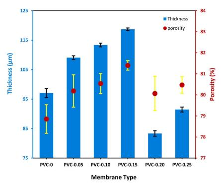
Fig. 10 PVC/SiO<sub>2</sub>-SDS MMMs porosity and thickness compared with the pristine membrane.
