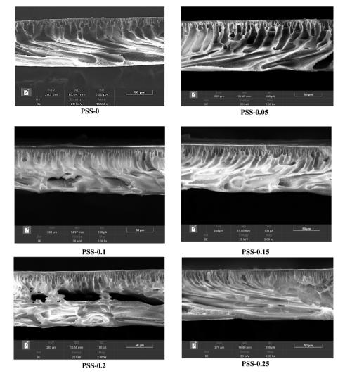
SEM of the cross-sectional structure of the pristine membrane and MMMs.
