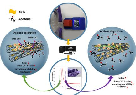
**Synergistic sensing properties of a standalone portable prototype using an integrated graphitic carbon nitride–carbon nanotube film for ultra-sensitive and selective acetone detection**
