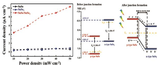
**Construction of a SnSe/SnSe<sub>2</sub> heterojunction for superior photoelectrochemical photodetectors**
