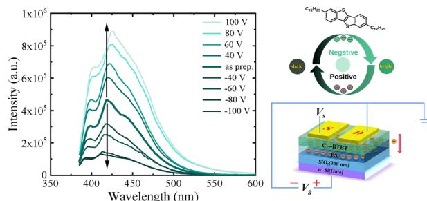
**Space charge-induced electrofluorochromic behavior for  $C_{12}$ -BTBT-based thin-film devices**
