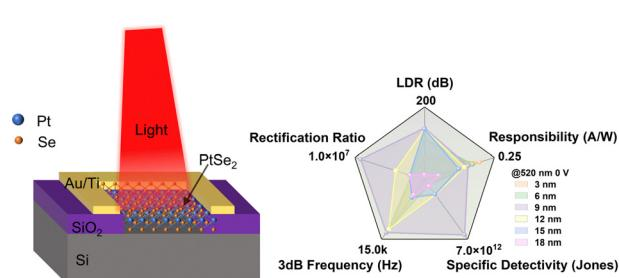
**PtSe<sub>2</sub> thickness engineering towards fast response, large linear dynamic range, and broadband PtSe<sub>2</sub>/Si heterojunction photodetectors**
