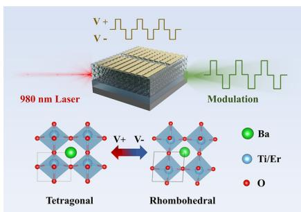
**Bidirectional luminescence modulation of BTO:Yb/Er ferroelectric films based on phase transition**
