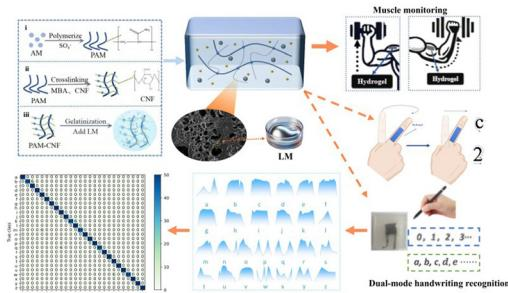
**A multifunctional, double network cellulose-acrylamide based hydrogel sensor reinforced using a liquid metal for human motion detection and dual-mode handwriting recognition via a transfer learning algorithm**
