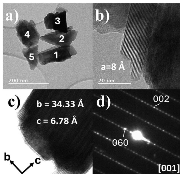
**Fig. 4** (a) TEM micrograph of five grains from KNNs thin films deposited using a stoichiometric commercial target, which were analyzed by EDXS. (b) and (c) TEM images and (d) electron diffraction pattern of K<sub>4</sub>Nb<sub>6</sub>O<sub>17</sub> phase along the [001] zone axis.
