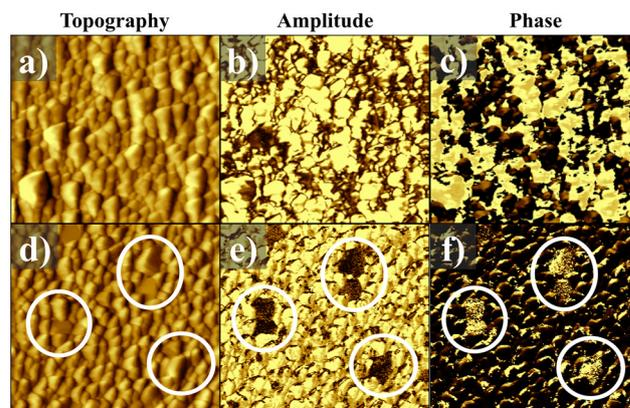
Fig. 6 Topography, amplitude and phase images from  $2 \times 2 \mu\text{m}^2$  area of (a)–(c) KNNe and (d)–(f) KNNs thin films obtained using an enriched target and a stoichiometric commercial target, respectively. White circles enclose flat grains, which present non-piezoelectric response.
