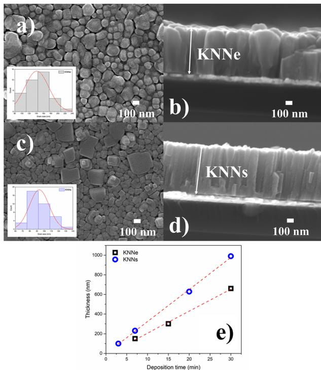
**Fig. 3** Surface and cross-section SEM micrographs of (a) and (b) KNNe, and (c) and (d) KNNs thin films deposited using a K-enriched target and a stoichiometric commercial target, respectively. Histograms of the grain size distribution are shown as inset in each surface micrograph. (e) Deposition ratio of KNNe and KNNs thin films.
