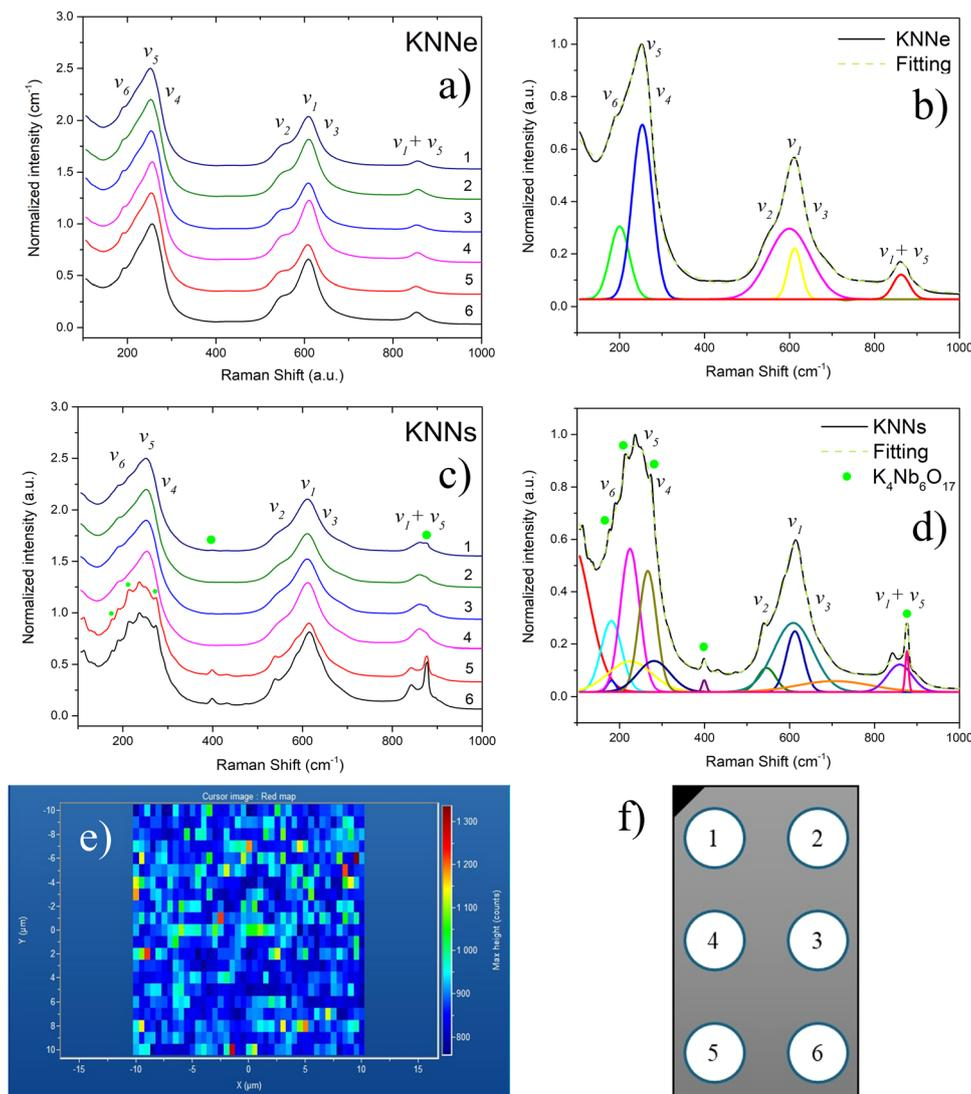
Fig. 2 Raman spectra mapping and deconvolution of (a) and (b) KNNe and (c) and (d) KNNs thin films obtained using an enriched target and a stoichiometric commercial target, respectively. (e) Raman mapping of KNNs recording in zone 5, the color code indicates an intense signal of the  $K_4Nb_6O_{17}$  secondary phase in red and weak signal in blue. (f) Scheme of the thin film and the areas analyzed by Raman on a  $10 \times 20 \text{ mm}^2$  substrate.
