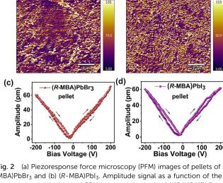
Fig. 2 (a) Piezoresponse force microscopy (PFM) images of pellets of (R-MBA)PbBr<sub>3</sub> and (b) (R-MBA)PbI<sub>3</sub>. Amplitude signal as a function of the tip bias, representing the local PFM hysteresis loops for (c) (R-MBA)PbBr<sub>3</sub> and (d) (R-MBA)PbI<sub>3</sub> pellets.
