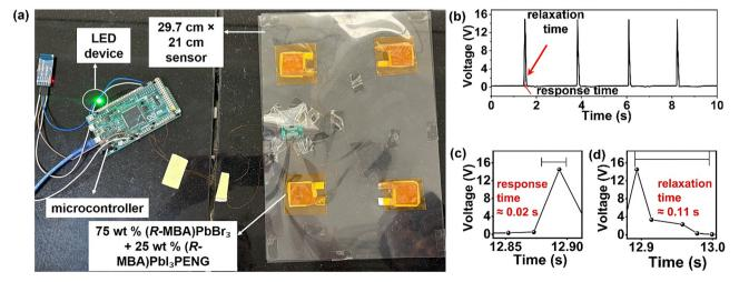
Fig. 5 (a) Photograph of the assembled sensor with four 15 wt% high-performing PENG devices between polyethylene terephthalate (PET) sheets. (b) Rectified voltage responses generated by the self-powered sensor during hand-tapping loading and unloading cycles. (c) and (d) Enlarged view of the curves in panel (b), showing the response and relaxation times, respectively
