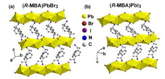
Fig. 1 Crystal structure diagrams of (a) (R-MBA)PbBrz and (b) (R-MBA)PbIz obtained from SCXRD data at 100 K. The structure comprises onedimensional chains of lead-halide octahedra with R-MBA cations positioned between them.
