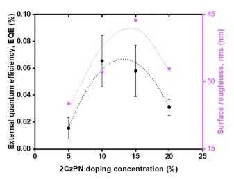
Fig. 3 (left y-axis) External quantum efficiency (at  $V_{\rm ds} = V_{\rm gate} = -100$  V) and (right y-axis) surface roughness of the topmost deposited layer (DFH-4T) as a function of different 2CzPN doping concentrations within the emissive blend for **3L-OLET**. Dashed lines are a guide-to-the-eye only.
