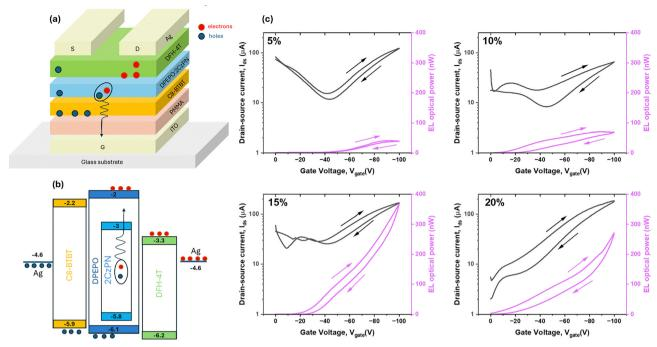
Fig. 2 (a) Simplified schematic of the multilayer transistor heterostructure and (b) its energy levels. (c) Saturation transfer curves ( $I_{ds}$  vs.  $V_{qate}@V_{ds} = I_{qate}$ -100 V) for **3L-OLET** with a DPEPO:2CzPN emissive layer with 2CzPN doping concentrations of 5, 10, 15, and 20%. The right y-axis refers to the electroluminescence light output (EL) measured through the gate electrode. Direction of sweeps is also indicated.
