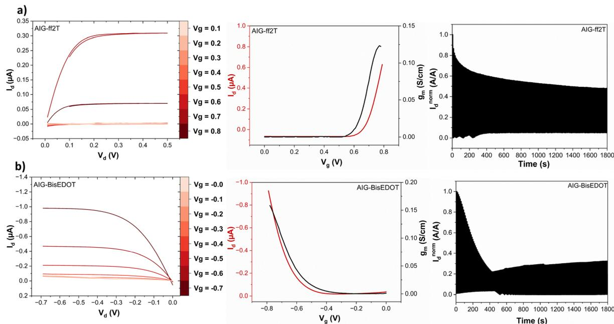
Fig. 3 Output (left), transfer and normalised transconductance (middle), and cycling stability (right) plots for OECTs with (a) **AIG-ff2T**, and (b) **AIG-bisEDOT** active materials at  $V_d = -0.4$  V for p-type (**AIG-bisEDOT**) and  $V_d = 0.4$  V for n-type (**AIG-ff2T**). Transfer and output curves were collected at  $0.1 \text{ Vs}^{-1}$ .
