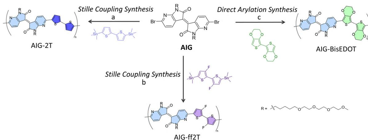
**Scheme 1** Synthesis and chemical structures of the azaisoindigo-based polymers with amphiphathic sidechains. (a)  $\text{Pd}_2(\text{dba})_3$ ,  $\text{P}(\text{o-tol})_3$ , 110 °C, Toluene/DMF, 24 h, (b)  $\text{Pd}_2(\text{dba})_3$ ,  $\text{P}(\text{o-tol})_3$ , 110 °C, Toluene, 24 h, (c)  $\text{Pd}(\text{OAc})_2$ , tris(2-methoxyphenyl)phosphine,  $\text{Cs}_2\text{CO}_3$ , caesium pivalate, 120 °C, chlorobenzene, 30 h.
