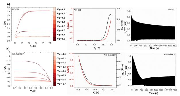
Fig. 3 Output (left), transfer and normalised transconductance (middle), and cycling stability (right) plots for OECTs with (a) AIG-ff2T, and (b) **AIG-bisEDOT** active materials at  $V_d = -0.4$  V for p-type (**AIG-bisEDOT**) and  $V_d = 0.4$  V for n-type (**AIG-ff2T**). Transfer and output curves were collected at 0.1 Vs<sup>-1</sup>
