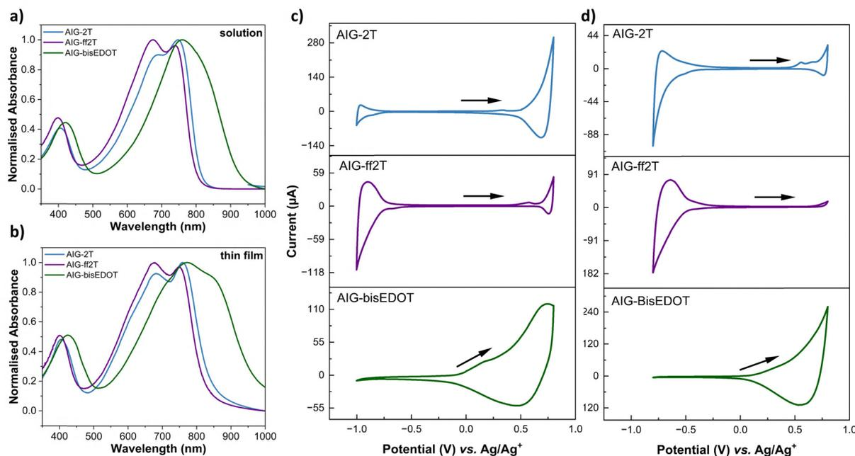
Fig. 1 Normalised UV-Vis-NIR spectra of the polymers in (a) chloroform solution and (b) thin films; cyclic voltammograms of thin films recorded in (c) acetonitrile solution of 0.1 M TBAPF<sub>6</sub> at a scan rate of 100 mV s<sup>-1</sup> and in (d) 0.1 M NaCl aqueous solution at a scan rate of 50 mV s<sup>-1</sup>.
