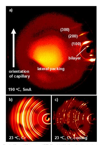
Fig. 4 2D vt pXRD images of BF3-Cl at (a) 190 °C on first heating in the SmA phase showing its propensity for spontaneous alignment; (b) 23 °C in the crystalline phase obtained by precipitation from solution; and (c) 23  $^{\circ}$ C on cooling into the crystalline phase obtained by crystallization from the aligned SmA phase. The intense diffraction spots in the diffraction pattern of (c) indicate the formation of larger crystalline domains than by crystallisation from solution in (b).
