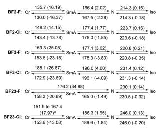
Fig. 6 Phase transition temperatures (°C) and (enthalpies (kJ mol<sup>-1</sup>)) of derivatives with the inner benzene ring (B) partially fluorinated. Values are determined by DSC at 5 °C min<sup>-1</sup> under N<sub>2</sub> for 2nd-heating and 1stcooling runs. Cr = crystalline phase; SmA = smectic A; N = nematic; Iso = isotropic liquid. <sup>a</sup> Broad melting event with several transitions; values given are the onsets of the transitions for the first and last thermal event.
