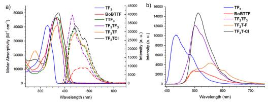
Fig. 10 Absorption and emission spectra of derivatives with the bithiophene moiety partially or fully fluorinated in (a) CH<sub>2</sub>Cl<sub>2</sub> and (b) as thin films sandwiched between quartz slides.  $\lambda_{\rm Exc}$  = 365 nm for both
