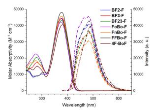
Fig. 11 Absorption and emission spectra of core-only calamitics with the inner benzene ring or benzoxazole's benzene ring partially or fully fluorinated in CH<sub>2</sub>Cl<sub>2</sub>. ( $\lambda_{Exc}$  = 365 nm).
