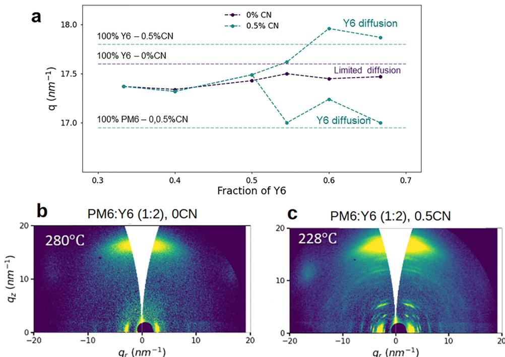
**Fig. 3** (a)  $q$ -position(s) of the  $\pi$ - $\pi$  stacking peak(s) maximum from GIWAXS of PM6:Y6 thin films with different donor:acceptor ratios, deposited from a chloroform solution without (0%) or with (0.5%) 1-chloronaphthalene (CN). The dashed horizontal lines represent the  $q$ -positions of this peak for the patterns of the single components PM6 and Y6 (0% and 0.5% CN). (b) and (c) GIWAXS patterns from Y6-rich samples at high temperature, (b) without and (c) with 1-chloronaphthalene.
