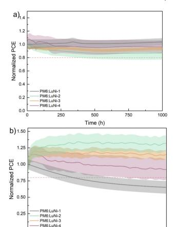
Fig. 3 Variation of normalized PCE of the relevant devices. (a) Thermal stability of the devices based on PM6:LuNi-1, PM6:LuNi-2, PM6:LuNi-3, and PM6:LuNi-4 baked in an oven at 65 °C, (b) photostability devices based on PM6:LuNi-1, PM6:LuNi-2, PM6:LuNi-3, and PM6:LuNi-4 measured under one sun illumination in ambient humidity at room temperature (The continuous line represents the average and the colored bands represent the standard deviation of 8 pixels)
