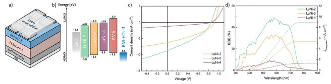
Fig. 2 (a) Scheme of an inverted device, (b) energy diagram of LuNi-2, LuNi-3, LuNi-4 thin film compared to ZnO, BM-HTL-1 and PM6 materials, (c) J-V curves and (d) EQE curves of the best performing pixels.
