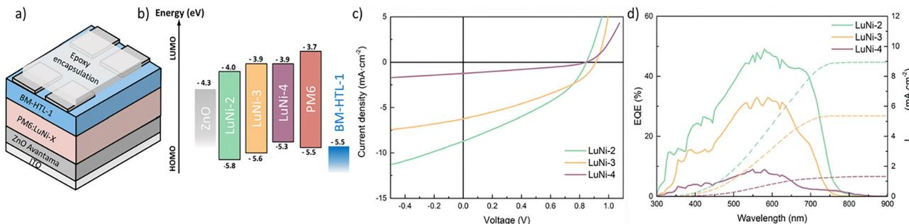
Fig. 2 (a) Scheme of an inverted device, (b) energy diagram of **LuNi-2**, **LuNi-3**, **LuNi-4** thin film compared to ZnO, BM-HTL-1 and PM6 materials, (c)  $J$ - $V$  curves and (d) EQE curves of the best performing pixels.
