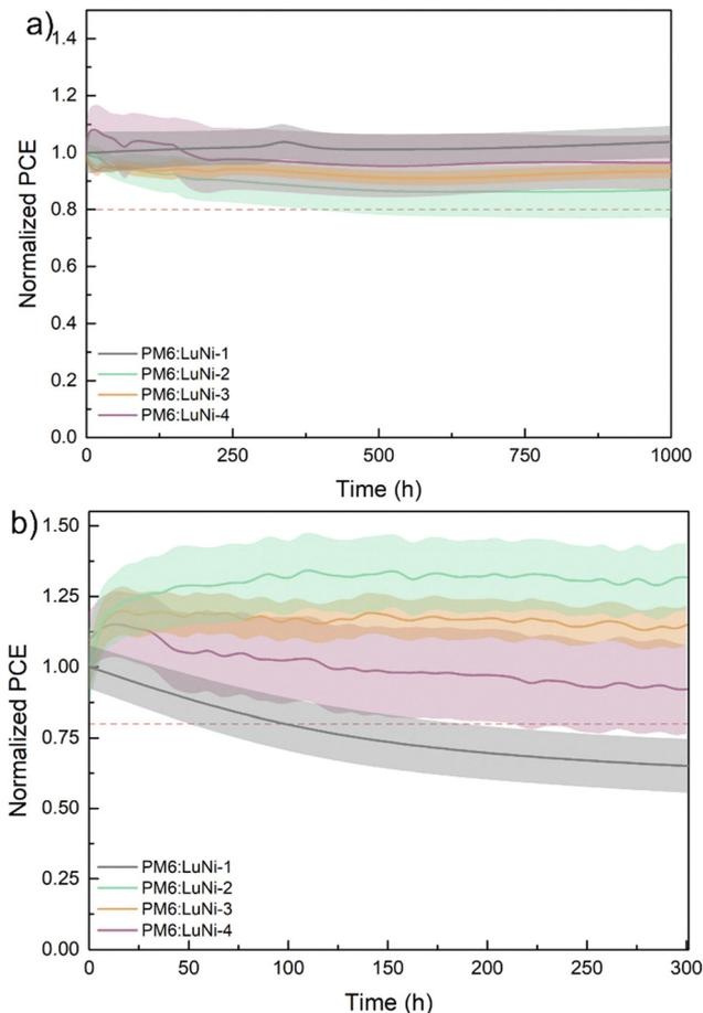
Fig. 3 Variation of normalized PCE of the relevant devices. (a) Thermal stability of the devices based on **PM6:LuNi-1**, **PM6:LuNi-2**, **PM6:LuNi-3**, and **PM6:LuNi-4** baked in an oven at 65 °C, (b) photostability devices based on **PM6:LuNi-1**, **PM6:LuNi-2**, **PM6:LuNi-3**, and **PM6:LuNi-4** measured under one sun illumination in ambient humidity at room temperature (The continuous line represents the average and the colored bands represent the standard deviation of 8 pixels).
