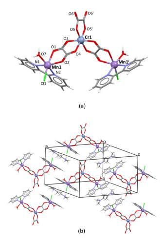
Fig. 1 (a) Heterotrinucler anion  $[\{Mn(bpy)(H_2O)Cl(\mu-C_2O_4)\}_2Cr(C_2O_4)]^-$  in compound 1, related by the symmetry operator (i) 1 - x, y, 1/2 - z; (b) crystal packing of cations and anions in the (101) plane.
