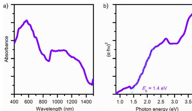
**Fig. 10** Optical properties of  $\text{Mn}_2\text{CrO}_4$  prepared by thermal decomposition of **1** at  $900\text{ }^\circ\text{C}$ : (a) Kubelka–Munk diffuse reflectance absorption spectrum; (b) Tauc's plot corresponding to direct transition; the dashed red line indicates the band gap energy.
