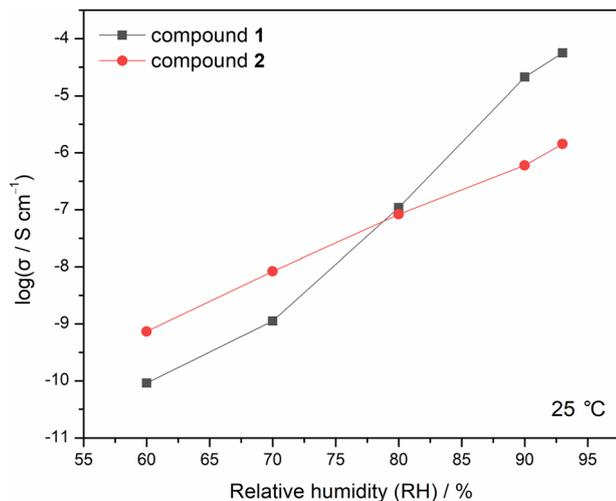
Fig. 3 The proton conductivity as a function of RH at room temperature of compounds  $[\text{NH}(\text{CH}_3)_2(\text{C}_2\text{H}_5)][\text{Mn}_2\text{Cr}(\text{bpy})_2(\text{H}_2\text{O})_2\text{Cl}_2(\text{C}_2\text{O}_4)_3]$  (**1**) and  $[\text{NH}(\text{CH}_3)(\text{C}_2\text{H}_5)_2][\text{Mn}_2\text{Cr}(\text{bpy})_2(\text{H}_2\text{O})_2\text{Cl}_2(\text{C}_2\text{O}_4)_3]$  (**2**).
