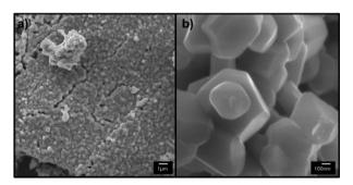
Fig. 9 Low (a) and high (b) magnification SEM images of Mn<sub>2</sub>CrO<sub>4</sub> oxide prepared using the molecular precursor route at 900 °C.
