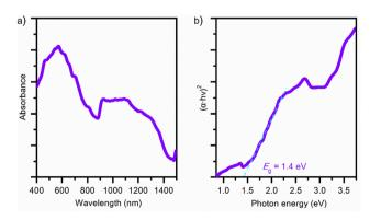
Fig. 10 Optical properties of Mn<sub>2</sub>CrO<sub>4</sub> prepared by thermal decomposition of 1 at 900 °C: (a) Kubelka-Munk diffuse reflectance absorption spectrum; (b) Tauc's plot corresponding to direct transition; the dashed red line indicates the band gap energy.
