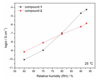
Fig. 3 The proton conductivity as a function of RH at room temperature of compounds  $[NH(CH_3)_2(C_2H_5)][Mn_2Cr(bpy)_2(H_2O)_2Cl_2(C_2O_4)_3]$  (1) and  $[NH(CH_3)(C_2H_5)_2][Mn_2Cr(bpy)_2(H_2O)_2Cl_2(C_2O_4)_3]$  (2).
