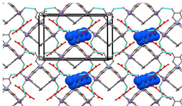
Fig. 2 Crystal packing in the (001) plane achieved through hydrogen bonds between anions (cyan sticks) in compound **1**. Disordered cations are depicted in red. The structure contains voids (depicted in blue) running perpendicular to the hydrogen bonding network in the (001) plane.
