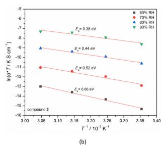
Fig. 4 Arrhenius-type plots of the temperature dependence of the DC conductivity with the corresponding value of activation energy for (a) compound 1 and (b) compound 2.
