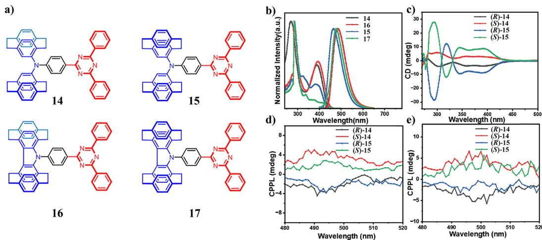
Fig. 7 (a) Schematic diagrams of **14**, **15**, **16** and **17**. (b) Normalized UV/Vis absorption and PL spectra of **14**, **15**, **16** and **17**. (c) CD of *R/S*-**14** and *R/S*-**15**. (d) CPPL spectra of *R/S*-**14** and *R/S*-**15** in toluene. (e) CPPL spectra of *R/S*-**14** and *R/S*-**15** in doped films 3 wt% in mCBP. Reproduced with permission from ref. 40. Copyright 2024, Wiley-VCH.
