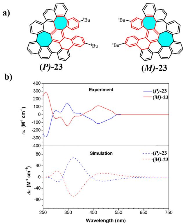
Fig. 10 (a) Schematic diagrams of (**P**)-**23** and (**M**)-**23**. (b) Experimental (solid lines) and TD-DFT simulated (dashed lines) CD spectra of (**P**)-**23** and (**M**)-**23**. Reproduced with permission from ref. 54. Copyright 2020, American Chemical Society.
