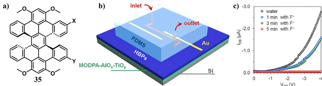
Fig. 21 (a) Schematic diagram of **35** ( $X = -(CH_2)_3CH_3$ ,  $Y = -(CH_2)_4OSi(CH_3)_3$ ). (b) Schematic drawing of the sensor combining a microchannel and a transistor channel of functionalized HBPs. (c) Transfer  $I$ - $V$  curves for the thin-film transistor of **35** as measured under deionized water and under an aqueous solution of KF (1 mM) for a certain period of time. Reproduced with permission from ref. 65. Copyright 2018, Elsevier.
