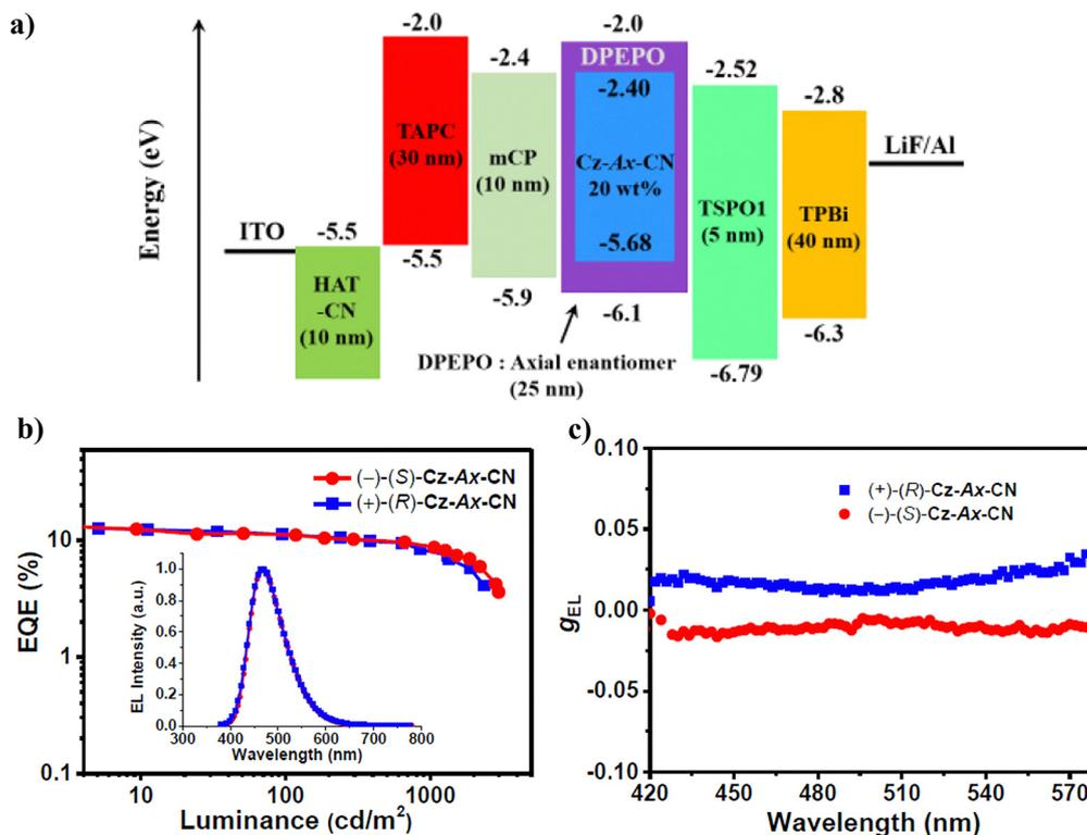
Fig. 17 (a) The energy diagram of CP-OLEDs based on (-)-(S)-**5** and (+)-(R)-**5**. (b) EQE–luminance characteristics. Inset: EL spectra of the devices at 6 V. (c) The  $g_{EL}$  values of the devices as a function of emission wavelength. Reproduced with permission from ref. 32. Copyright 2020, Wiley-VCH.
