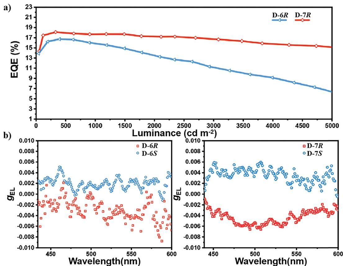
Fig. 18 (a) EQE luminance curves. (b)  $g_{EL}$ -wavelength curves of circularly polarized organic light-emitting diodes (CP-OLEDs) based on (*R/S*)-**6** and (*R/S*)-**7**. Reproduced with permission from ref. 33. Copyright 2021, Wiley-VCH.
