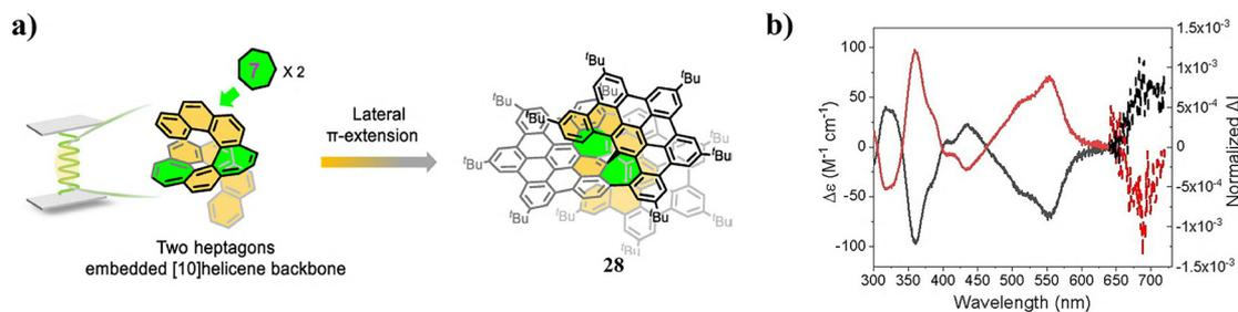
Fig. 13 (a) Schematic diagram of **28**. (b) Experimental ECD spectra (solid line) and experimental CPL spectra (dashed line, irradiation at 525 nm) of *P*-**28** (red) and *M*-**28** (black) (DCM at ca.  $1.6 \times 10^{-5}$  M and  $1.2 \times 10^{-5}$  M of *P*-**28** and *M*-**28**, respectively). Reproduced with permission from ref. 57. Copyright 2023, Wiley-VCH.
