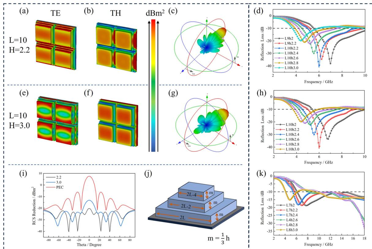
**Fig. 6** (a) and (e) TE, (b) and (f) TH polarization, (c) and (g) 3D RCS absorption of L10 h2.2 and L10 h3.0. (i) RCS reduction and (j) gradient structure design. Microwave absorption performance under different structural parameters ( $h = 2, 2.2, 2.4, 2.6, 2.8, 3.0$ ;  $L = 0, 1, 2, 3, 4, 5, 6, 7, 8, 9, 10$ ). (d) Optimal parameters for the small-band. (h) Lowest frequency for each thickness. (k) Maximum effective bandwidth for each thickness under different size parameters.
