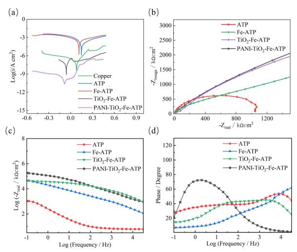
Fig. 7 (a) Tafel polarization curves of copper, ATP, Fe-ATP, TiO<sub>2</sub>-Fe-ATP and PANI-TiO<sub>2</sub>-Fe-ATP. (b) Nyquist plots, (c) impedance moduli and (d) phase angle plots of ATP, Fe-ATP, TiO<sub>2</sub>-Fe-ATP and PANI-TiO<sub>2</sub>-Fe-ATP
