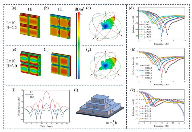
Fig. 6 (a) and (e) TE, (b) and (f) TH polarization, (c) and (g) 3D RCS absorption of L10 h2.2 and L10 h3.0. (i) RCS reduction and (j) gradient structure design. Microwave absorption performance under different structural parameters (h = 2, 2.2, 2.4, 2.6, 2.8, 3.0; L = 0, 1, 2, 3, 4, 5, 6, 7, 8, 9, 10). (d) Optimal parameters for the small-band. (h) Lowest frequency for each thickness. (k) Maximum effective bandwidth for each thickness under different size
