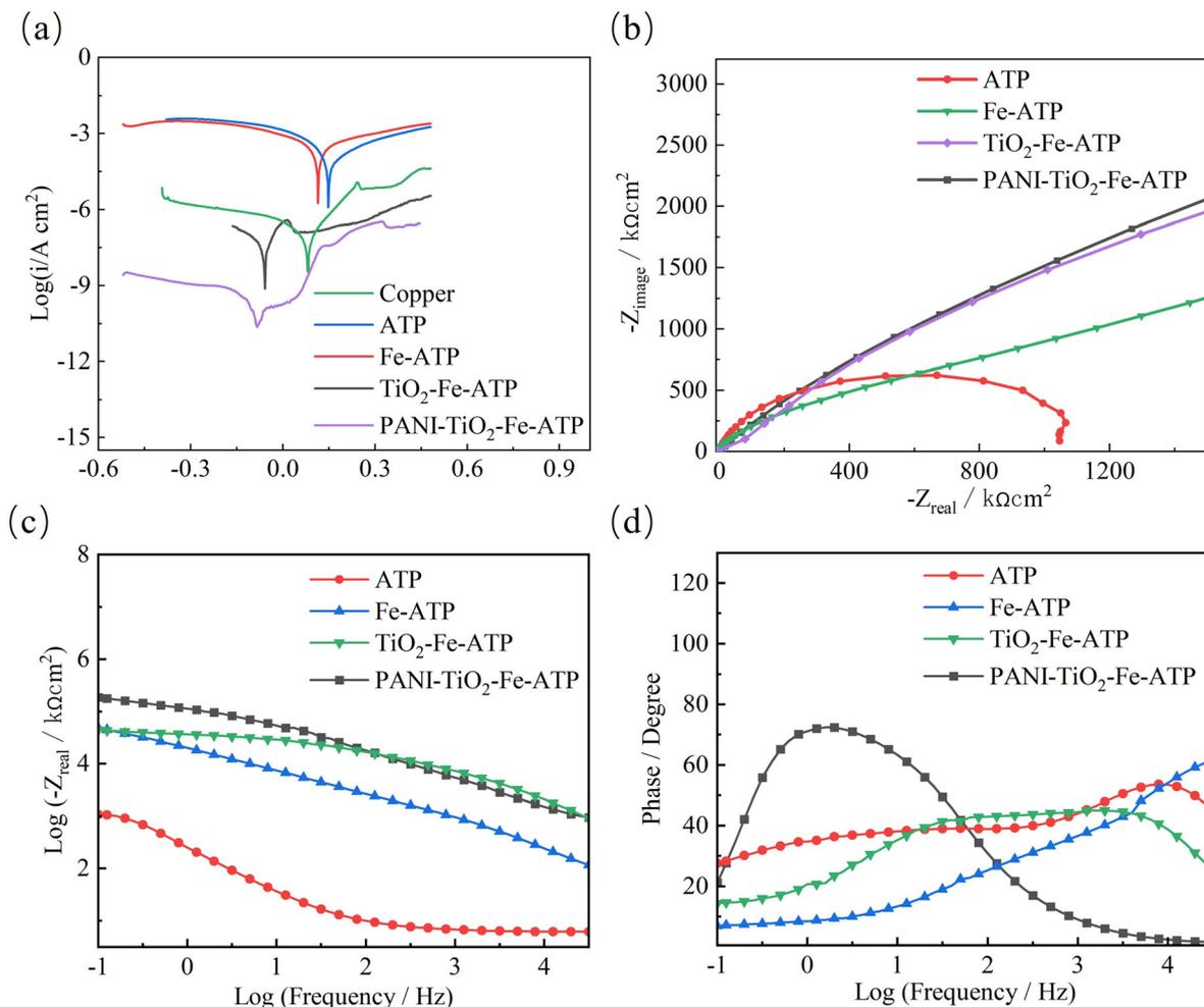
Fig. 7 (a) Tafel polarization curves of copper, ATP, Fe-ATP, TiO<sub>2</sub>-Fe-ATP and PANI-TiO<sub>2</sub>-Fe-ATP. (b) Nyquist plots, (c) impedance moduli and (d) phase angle plots of ATP, Fe-ATP, TiO<sub>2</sub>-Fe-ATP and PANI-TiO<sub>2</sub>-Fe-ATP.
