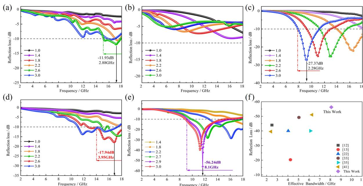
Fig. 4 Electromagnetic wave absorption performance. Reflection loss (RL) curves of (a) ATP, (b) Fe–ATP, (c) PANI–ATP, (d) TiO<sub>2</sub>–Fe–ATP, and (e) PANI–TiO<sub>2</sub>–Fe–ATP. (f) Reflection loss and effective bandwidth performance comparison.<sup>12,13,22,33,35</sup>
