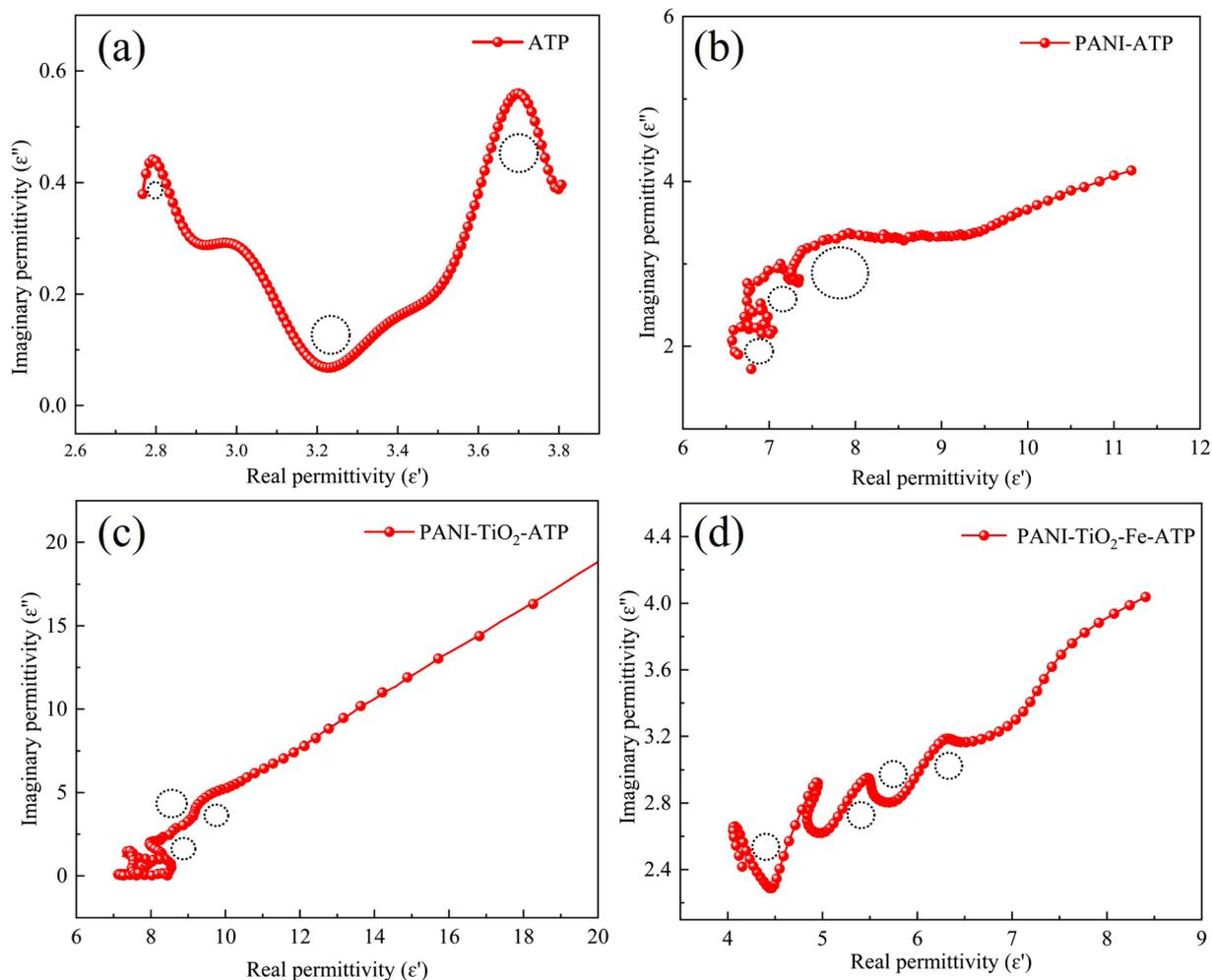
Fig. 3 Cole–Cole circles of (a) ATP, (b) PANI-ATP, (c) PANI-TiO<sub>2</sub>-ATP, and (d) PANI-TiO<sub>2</sub>-Fe-ATP.
