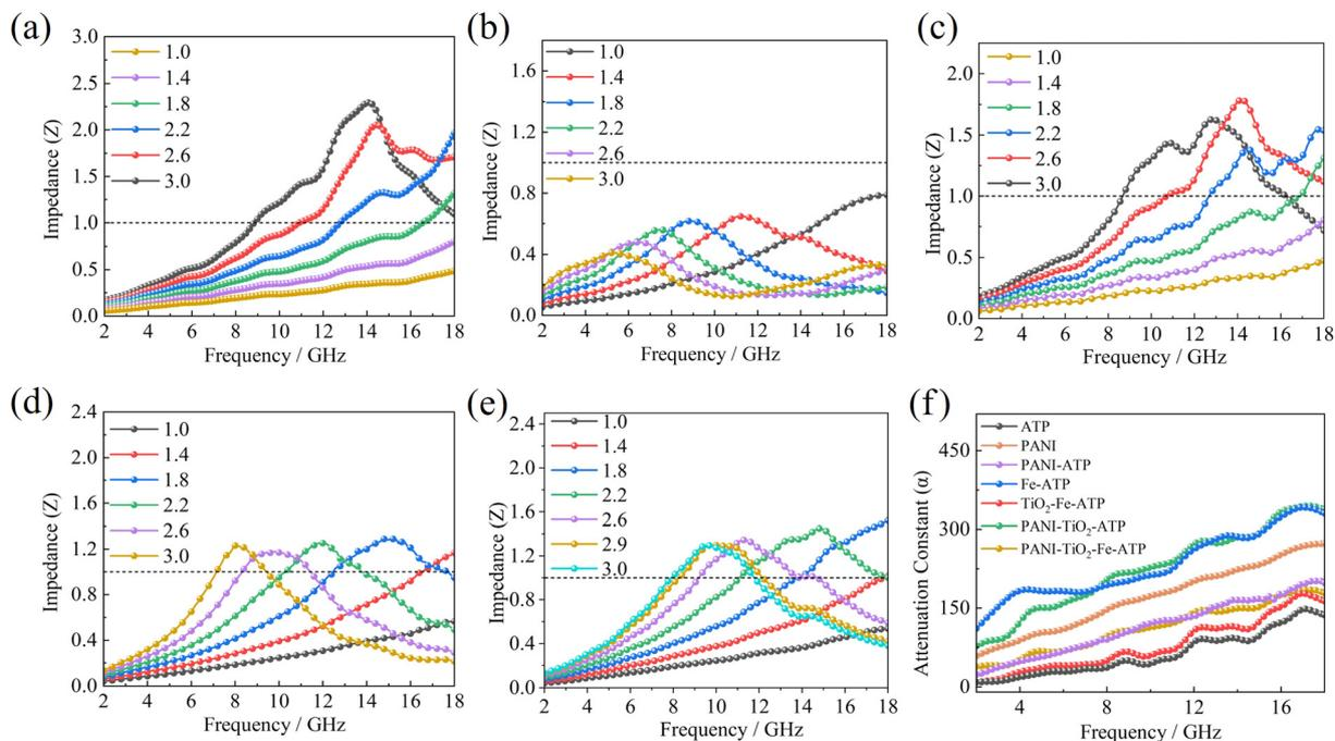
Fig. 5 Impedance match ( $Z$ ) curves of (a) ATP, (b) Fe-ATP, (c) TiO<sub>2</sub>-Fe-ATP, (d) PANI-ATP, and (e) PANI-TiO<sub>2</sub>-Fe-ATP and their (f) attenuation constant ( $\alpha$ ).
