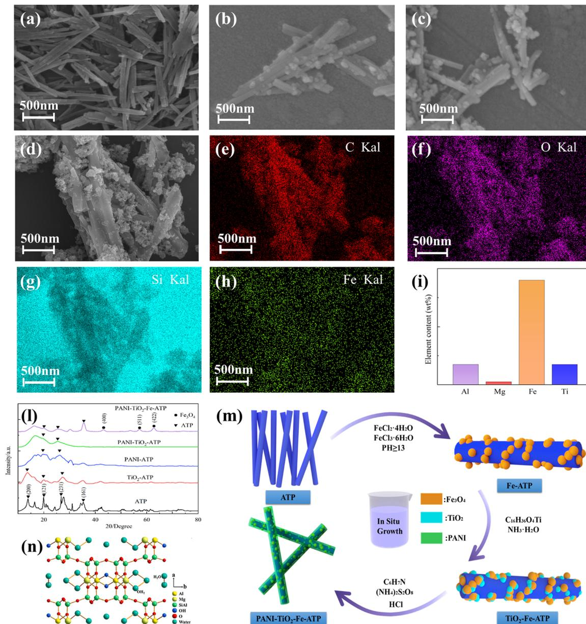
**Fig. 1** SEM images of (a) ATP, (b) Fe-ATP, (c) TiO<sub>2</sub>-Fe-ATP, and (d) PANI-TiO<sub>2</sub>-Fe-ATP. Elemental distribution profiles corresponding to PANI-TiO<sub>2</sub>-Fe-ATP of (e), (f), (g), (h) and (i) elemental contents of Al, Mg, Fe, and Ti. (j) XRD patterns. (m) Illustration of the synthesis process of PANI-TiO<sub>2</sub>-Fe-ATP. (n) Crystal structure of ATP.
