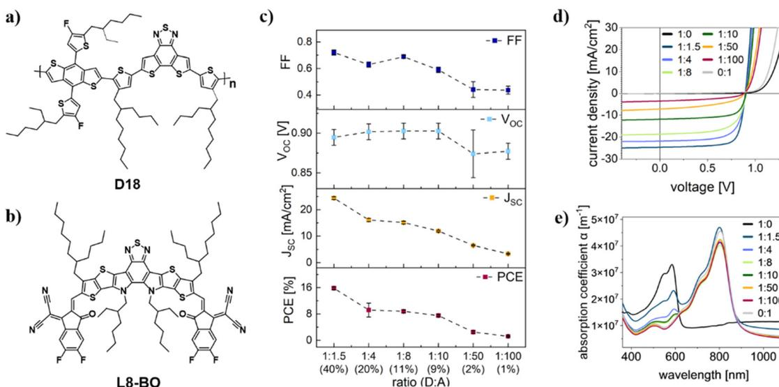
Fig. 1 Chemical structures of (a) D18, (b) L8-BO, (c) FF,  $V_{oc}$ ,  $J_{sc}$  and PCE plotted vs. the D:A ratio, (d)  $J$ - $V$  curves, measured under illumination, of solar cells with different D:A ratios and (e) their absorption spectra for the pure materials and the blends with different D18:L8-BO ratios from 1:1.5 to 1:100.
