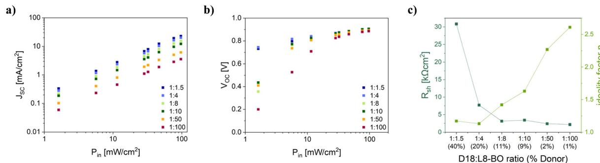
Fig. 6 Light intensity dependency of (a)  $J_{SC}$  and (b)  $V_{OC}$  of solar cells with different D18:L8-BO ratios and (c) shunt resistance ( $R_{sh}$ ) and ideality factors  $n$  of the solar cells with different D : A ratios.
