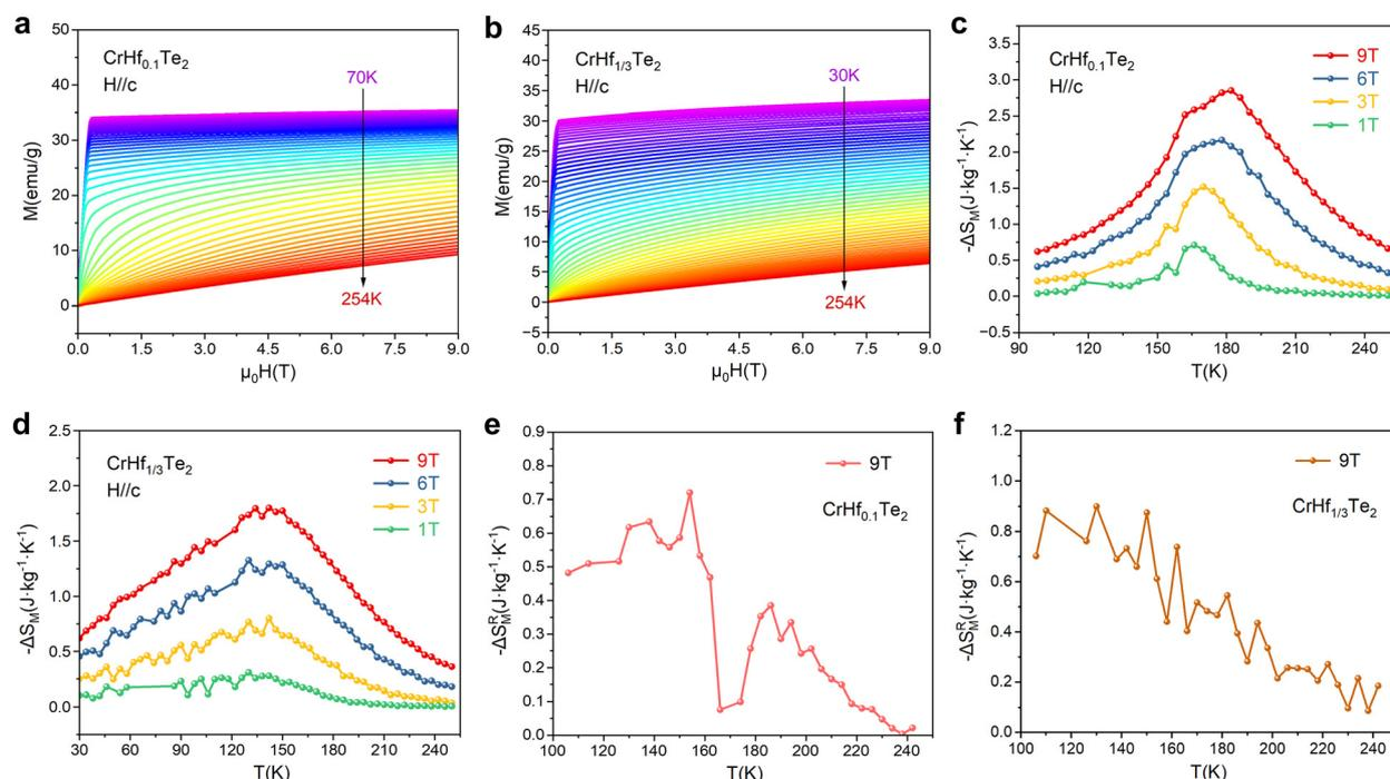
Fig. 3 (a) and (b) Isothermal field-dependent magnetization curves along the H//*c*-axis direction for CrHf<sub>0.1</sub>Te<sub>2</sub> and CrHf<sub>1/3</sub>Te<sub>2</sub>, respectively. (c) and (d) Curves of  $-\Delta S_M$  with temperature under a magnetic field parallel to the *c*-axis. (e) and (f) Rotating magnetic entropy changes of CrHf<sub>x</sub>Te<sub>2</sub> obtained by rotating from the *c*-axis to the *ab*-plane.
