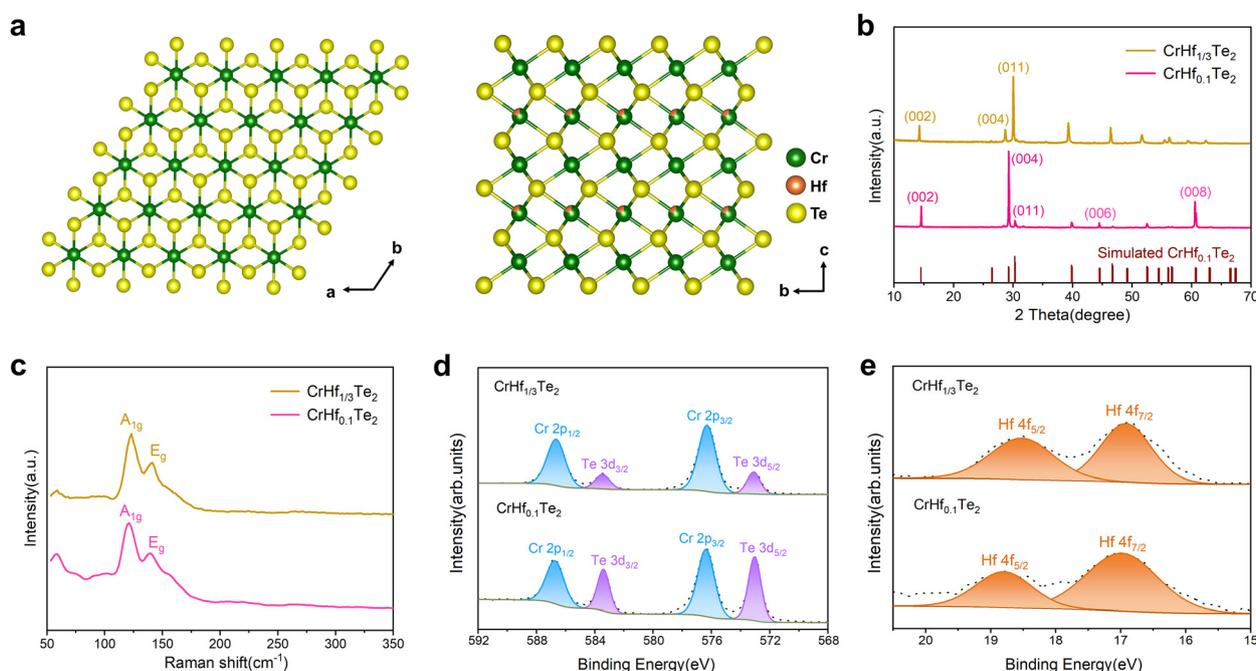
Fig. 1 (a) Crystal structure of trigonal  $\text{CrHf}_{0.1}\text{Te}_2$  viewed from the  $c$ -axis and  $a$ -axis. (b) PXRD patterns. (c) Raman spectra. (d) and (e) High-resolution XPS spectra of Cr 2p, Te 3d and Hf 4f for  $\text{CrHf}_x\text{Te}_2$  ( $x = 0.1, 1/3$ ).
