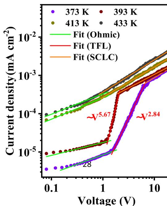
**Fig. 5** Temperature-dependent space charge limited current–voltage ( $J$ - $V$ ) characteristics of the Ag/FAPbBr<sub>2</sub>I SC/Ag device configuration at temperature  $T = 373$  K, 393 K, 413 K, and 433 K.
