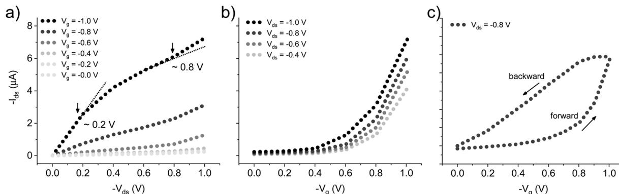
Fig. 4 (a) Output ( $-I_{ds}$  vs.  $-V_{ds}$  at selected  $V_g$  values), (b) transfer ( $-I_{ds}$  vs.  $-V_g$  at selected  $V_{ds}$  values) and (c) hysteresis transfer ( $-I_{ds}$  vs.  $-V_g$  at selected  $V_{ds}$  value in forward and backward directions) characteristics for P3HT-based OECT working with  $[C_{10}H_{21}SO_3Na]$  0.1 M electrolyte at 25 °C. The voltages at which the transistor output characteristic switches from linear to quasi-saturation regime are marked with arrows.
