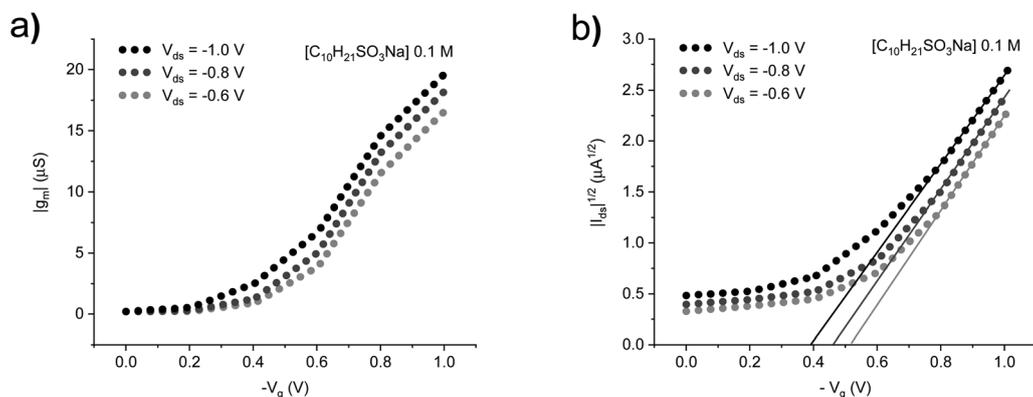
Fig. 5 (a) Transconductance ( $g_m$  vs.  $V_g$  at selected  $V_{ds}$  values) and (b) threshold voltage ( $|I_{ds}|^{1/2}$  vs.  $V_g$  at selected  $V_{ds}$  values) plots for P3HT-based OECT working with  $[C_{10}H_{21}SO_3Na]$  0.1 M electrolyte at 25 °C.
