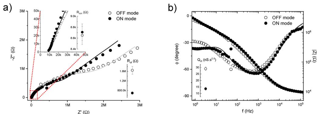
Fig. 6 (a) Nyquist and (b) Bode plots for P3HT-based OECT working with  $[C_{10}H_{21}SO_3Na]$  0.1 M electrolyte at 25 °C for different operation modes; i.e. OFF ( $V_{g,dc} = 0.0$  V) and ON ( $V_{g,dc} = -1.0$  V).
