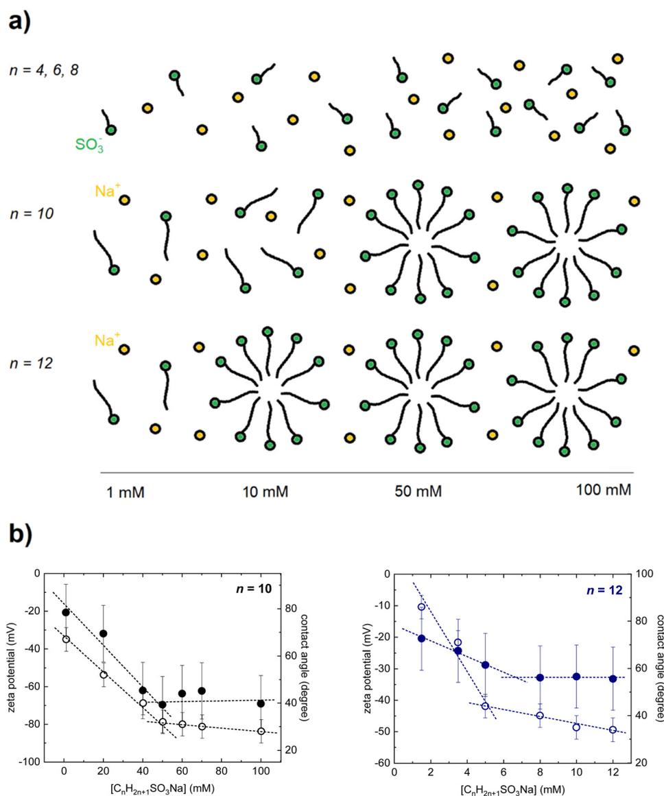
Fig. 1 (a) Schematization of critical micelle concentration for  $C_nH_{2n+1}SO_3Na$  ( $n = 4, 6, 8, 10$  and 12) and (b) zeta potential (full circles) and contact angle (hollow circles) at different  $C_nH_{2n+1}SO_3Na$  concentrations for  $n = 10$  and 12, at 25 and 30 °C, respectively.
