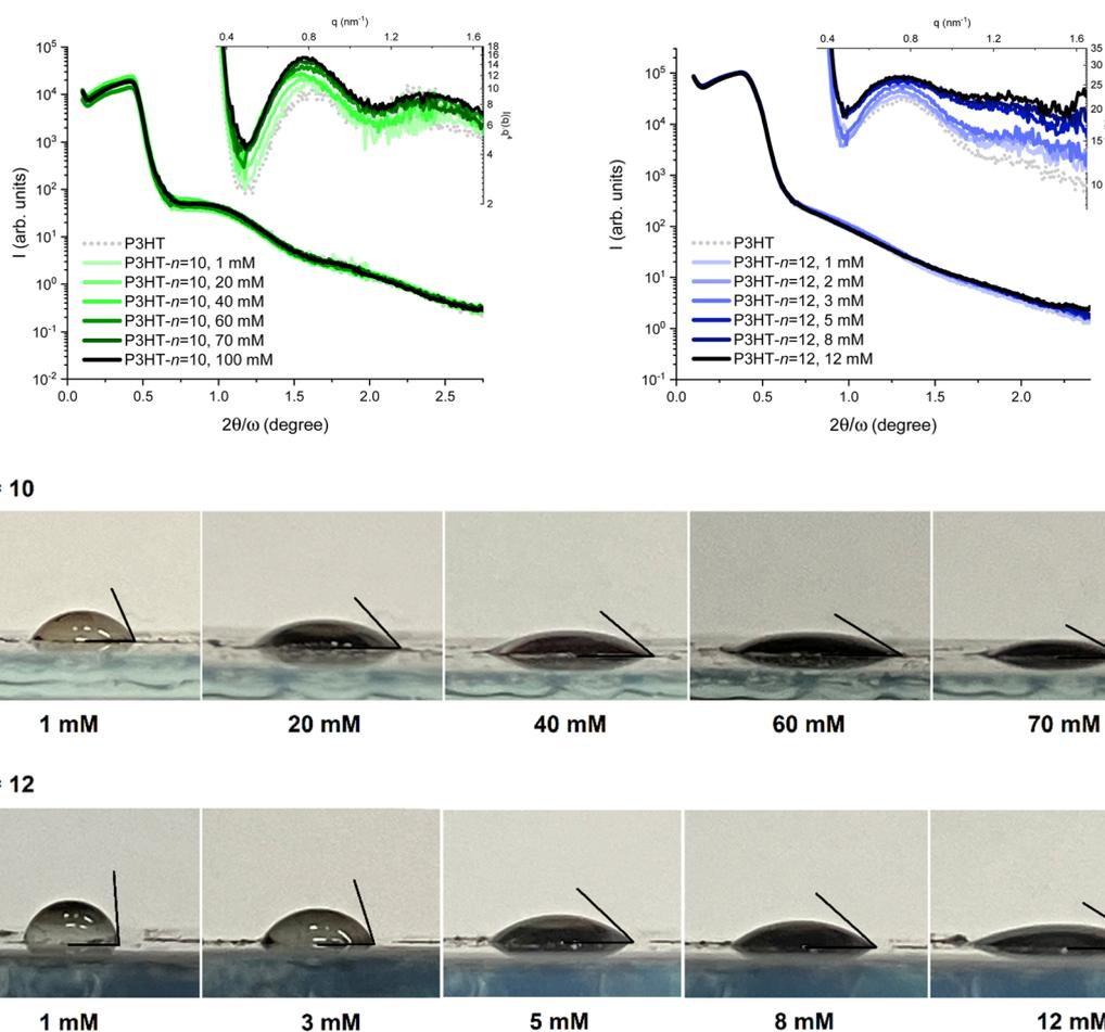
Fig. 2 X-ray reflectometry (XRR) curves depicted as  $I(q)$  vs.  $2\theta/\omega$  and  $I(q) \cdot q^4$  vs.  $q$  plots (upper panel) and contact angle images (lower panel) for P3HT films exposed at different  $C_nH_{2n+1}SO_3Na$  concentrations for  $n = 10$  and 12, at 25 and 30 °C, respectively.
