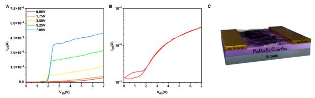
Fig. 4 Characteristic (a) output, (b) transfer curves for BGTC OTFTs prepared using P<sub>68</sub>D<sub>29</sub>S<sub>3</sub>-CL<sub>10</sub>-A<sub>25</sub> with sc-SWCNTs. The transfer curve was operated at a V<sub>SD</sub> of 3V, and the average of the last measurement of five transfer curves is presented to ensure the film is appropriately charged (c) BGTC device architecture.
