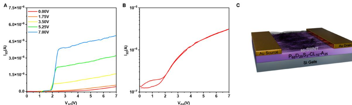
Fig. 4 Characteristic (a) output, (b) transfer curves for BGTC OTFTs prepared using  $P_{68}D_{29}S_3-CL_{10}-A_{25}$  with sc-SWCNTs. The transfer curve was operated at a  $V_{SD}$  of 3V, and the average of the last measurement of five transfer curves is presented to ensure the film is appropriately charged (c) BGTC device architecture.
