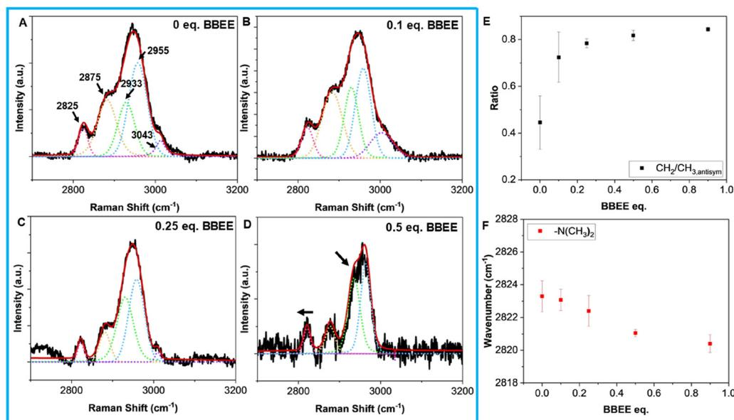
Fig. 2 (A)–(D) Raman spectra  $P_{50}D_{48}S_2-CL_Y-A_0$  crosslinking (black) together with the results of fitted peak analysis (red) of five mixed Lorentz–Gaussian functions (pink, yellow, green, blue, and purple) for 0, 0.1, 0.25, and 0.5 molar eq. BBEE to DMAEMA monomer units. (E)  $-CH_2/-CH_3$ , antisymmetric ratio and (F)  $-N(CH_3)_2$  Raman peak wavenumber plotted against BBEE molar equivalent to DMAEMA monomer units.
