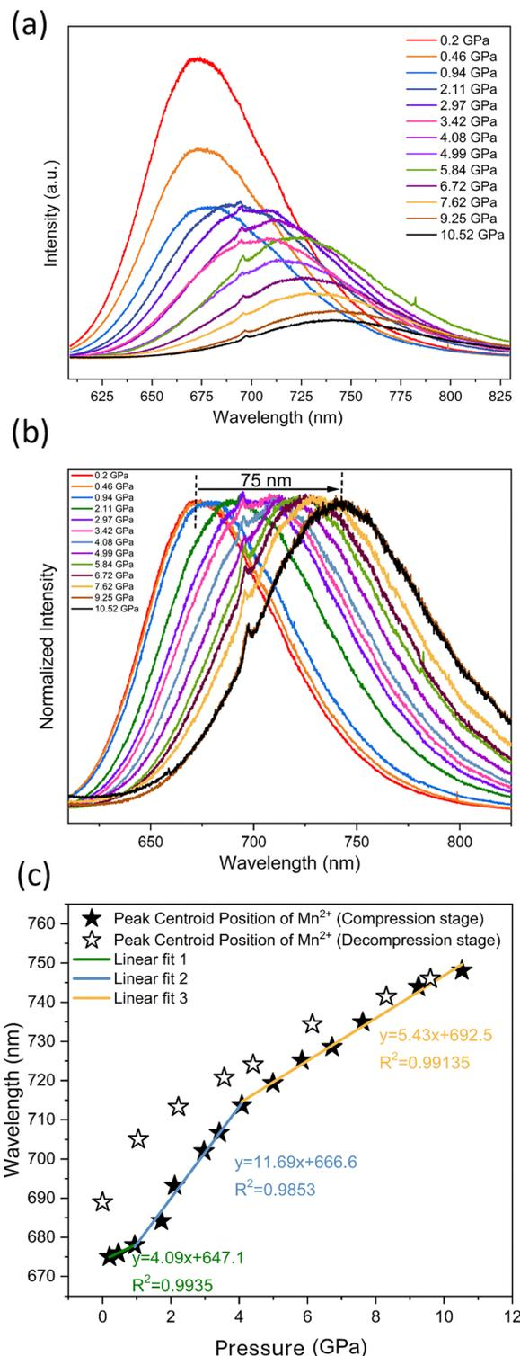
Fig. 6 *In situ* high-pressure compression PL spectra. (a) The emission spectra of MGO:Mn NPs excited at 360 nm. (b) Normalized emission spectra of MGO:Mn NPs excited at 360 nm. The sharp peaks here are from the ruby. (c) Linear regression fitting of emission positions during the compression stage. The emission centre of the decompression stage is included for comparison.
