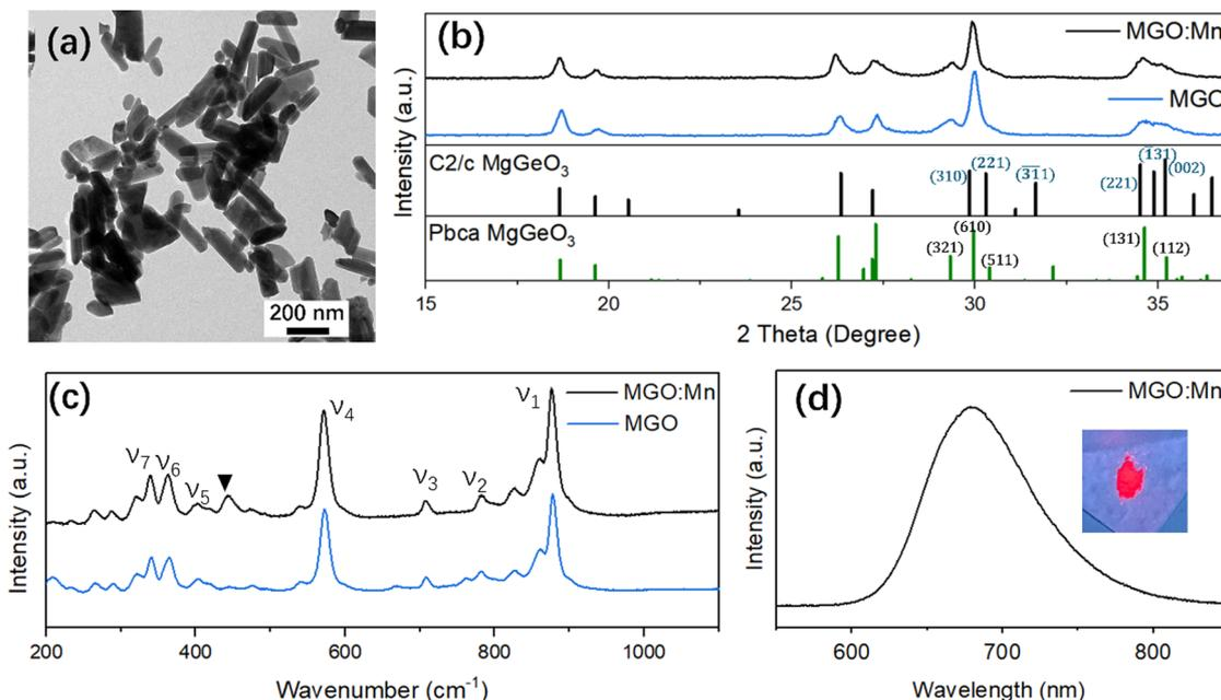
Fig. 2 (a) TEM image of MGO:Mn NPs. (b) XRD pattern of MGO:Mn (at ambient pressure). The standard patterns of  $C2/c$ <sup>30</sup> and  $Pbca$  (JCPDF 04-0008-8425)  $MgGeO_3$  were also included for comparison. (c) Raman spectra of MGO:Mn and MGO at ambient pressure. The prominent stretching bands from MGO were labelled. The solid triangle marked the stretching mode from  $GeO_2$ . (d) PL spectrum and optical photograph (inset) of MGO:Mn were recorded under 254 nm UV light excitation.
