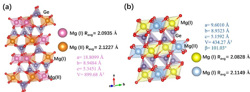
Fig. 1 Crystal structure of (a) *Pbca* and (b) *C2/c*  $\text{MgGeO}_3$ . Ge atoms are purple and O atoms are red. Colored octahedra represent Mg in different sites: pink: Mg(I) of *Pbca*  $\text{MgGeO}_3$ , orange: Mg(II) of *Pbca*  $\text{MgGeO}_3$ , yellow: Mg(I) of *C2/c*  $\text{MgGeO}_3$ , light blue: Mg(II) of *C2/c*  $\text{MgGeO}_3$ . The calculated average bond length for each  $\text{Mg}^{2+}$  site in *Pbca* and *C2/c* is listed above.
