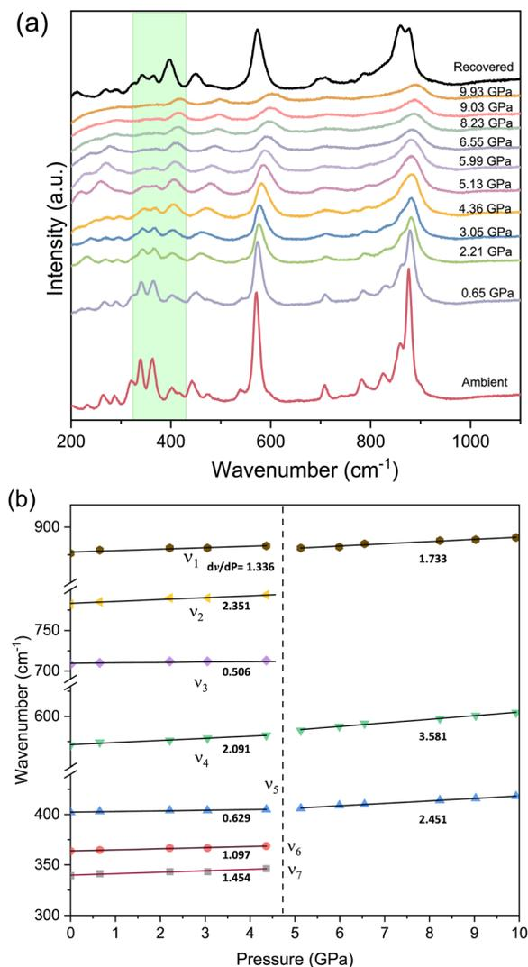
Fig. 3 (a) *In situ* high-pressure Raman spectra of MGO:Mn NPs measured at various pressure points during compression and after decompression. The shaded green area highlights the intensity change of  $\nu_5$  against  $\nu_6$  and  $\nu_7$  modes. (b) Pressure-dependence plot of selected Raman vibrational modes of MGO:Mn NPs for the compression data, with linear regression fits applied for each selected mode to determine the frequency shift rate.
