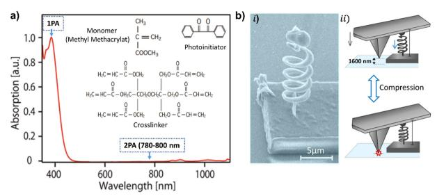
Fig. 8 (a) Absorption spectrum of MMA resin. The components of the resin are shown in the inset. (b) (i) SEM micrograph of a freestanding 2PP-printed nano-sized coil spring fabricated using the MMA resin shown in (a). (ii) Scheme illustrating a compression test performed on the μ-coil spring using AFM. (a) and (b) Reproduced under the terms of the Creative Commons License CC BY 4.0.<sup>109</sup> Copyright 2015, the Authors, published by Springer Nature.
