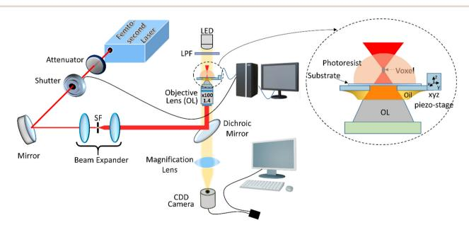
Fig. 10 Experimental setup for 2PP-assisted 3D nanoprinting. The setup is equipped with a three-axis PZT and inverted OL focusing configurations. SF: spatial filter, LPF: low pass filter
