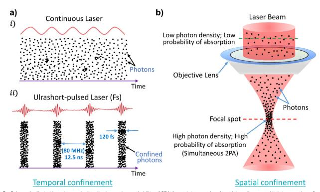
Fig. 5 Schematic illustrations demonstrating the increasing probability of 2PA through temporal and spatial confinement. High temporal confinement cannot be achieved by CW laser, which emits a continuously low photon density over time (ai). In contrast, Fs lasers, which emit high-instantaneous intensity pulses, can achieve high temporal confinement of photons (aii). (b) Spatial confinement of photons within an infinitely small volume (LFS) using a high-numerical OL.
